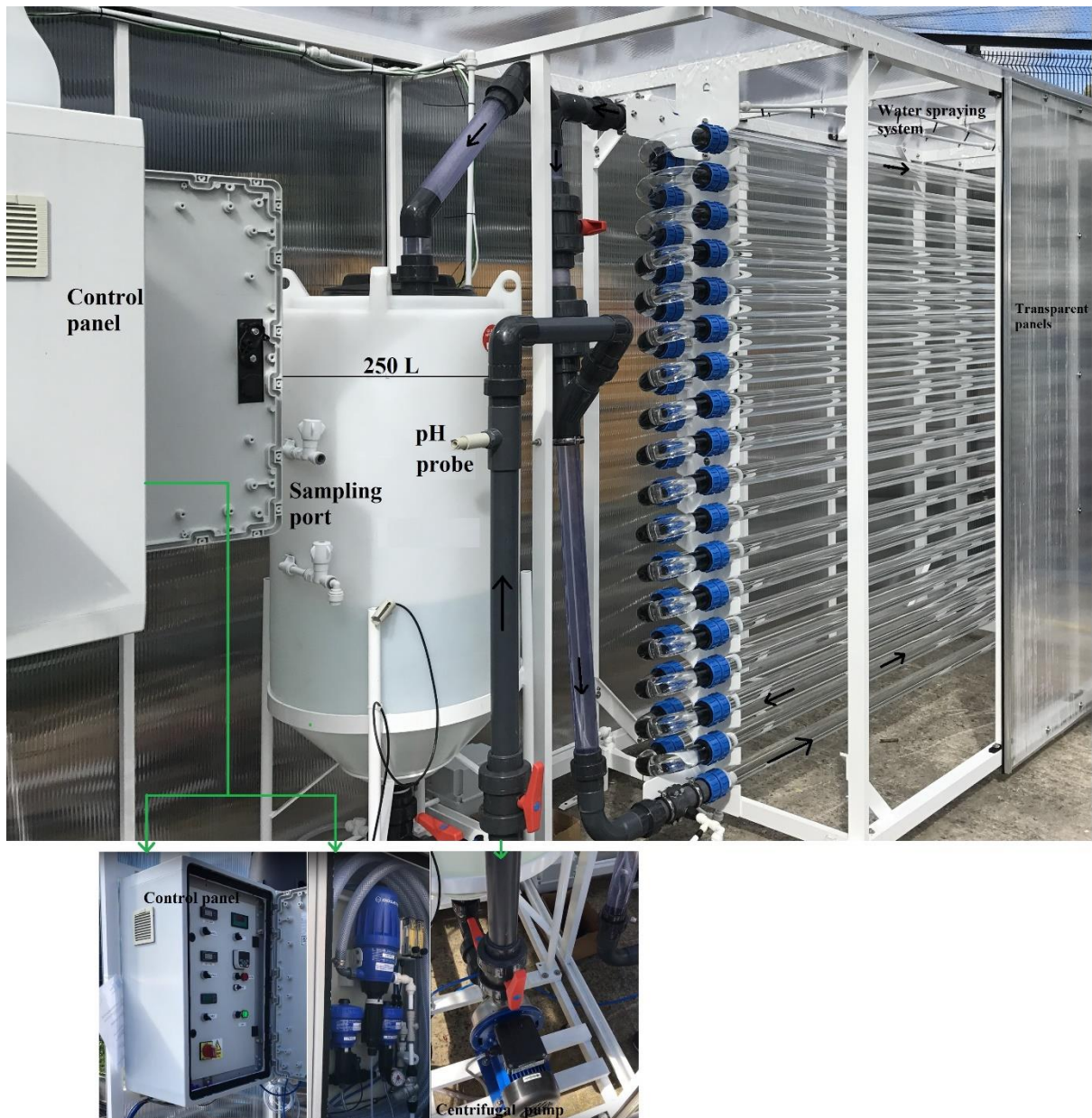
Figure 5.1: An outdoor 300 L PhycoFlow® Photobioreactor that was installed at Arthur Willis Environmental Centre (53.3832000157627° North, -1.4995194567741421° West), Department of Animal and Plant Sciences, University of Sheffield.
