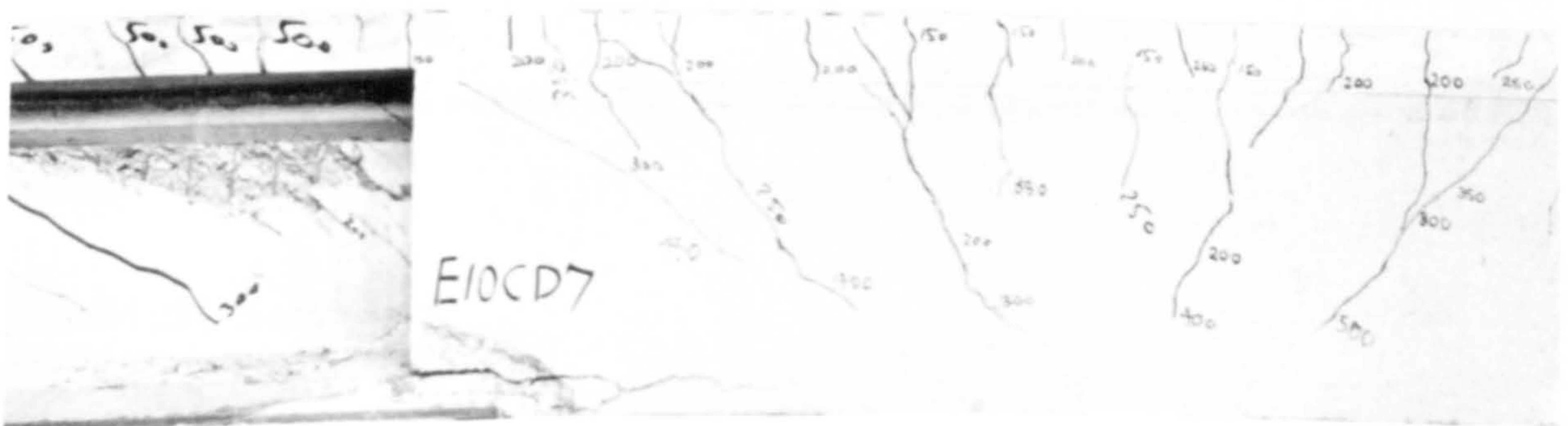
Plate 5.11 100mm Embedment Length (with Nib Stirrups) Condition in The Connection After Failure
