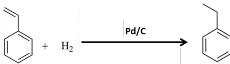
Figure 4.1: Reaction scheme for the hydrogenation of styrene to ethylbenzene.
