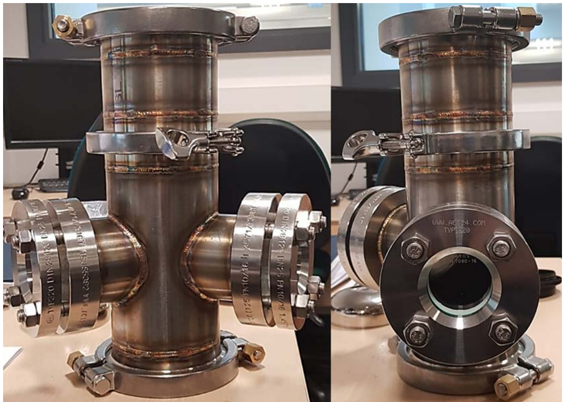
Figure 6.2: Images of pressurised falling film reactor showing the main body, the second top tube and the sight glass windows.
