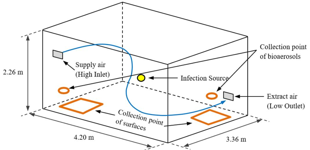
**Figure 7:1** The aerobiological chamber dimensions and the collection points of air and surfaces.
