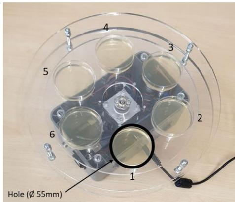
**Figure 6:2** Automated multiplate passive air sampler (AMPAS).
