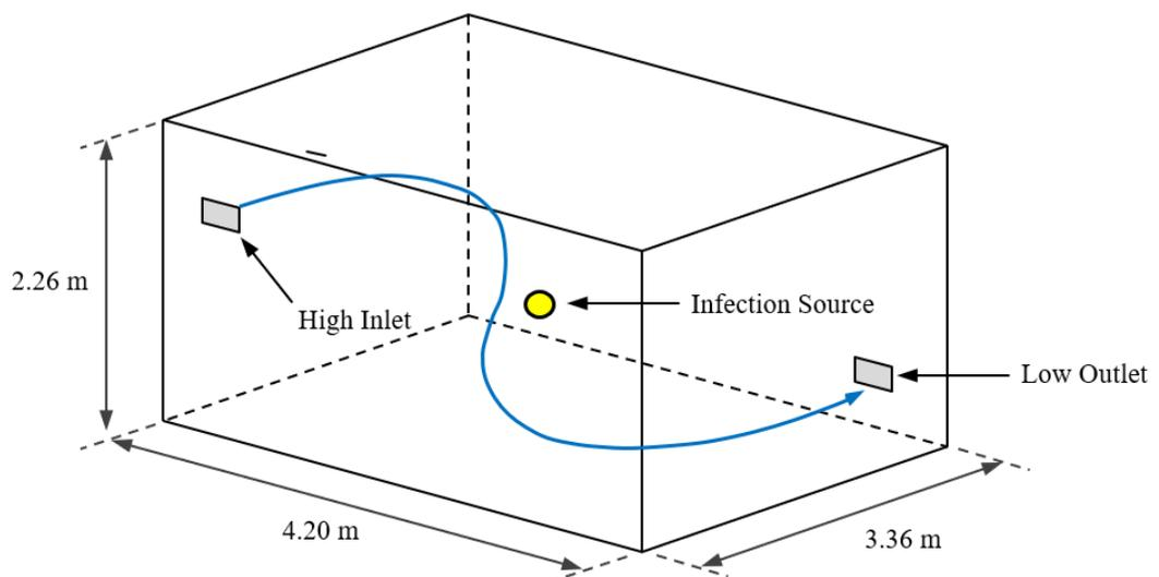
**Figure 6:6** The aerobiological chamber dimensions and ventilation
