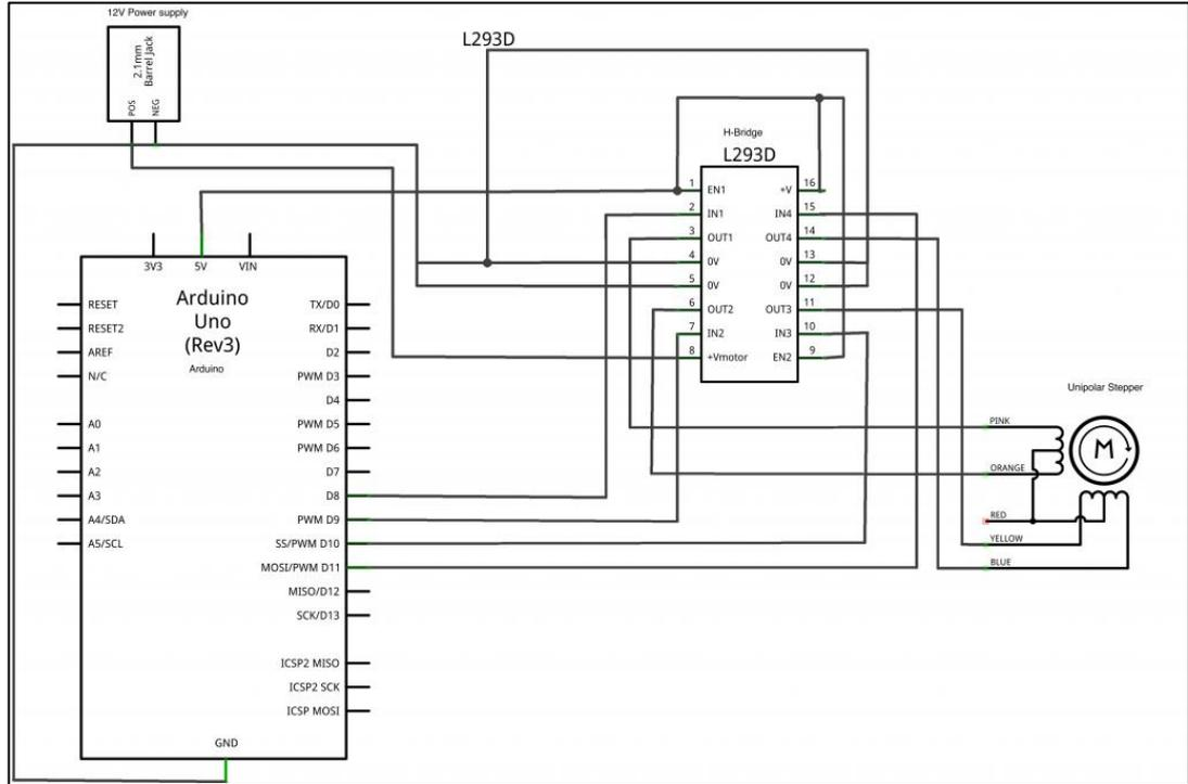
**Figure 6:1** Schematic drawing of an h-bridge and stepper motor connected to an Arduino, with the control wires added (Computing, 2020).
