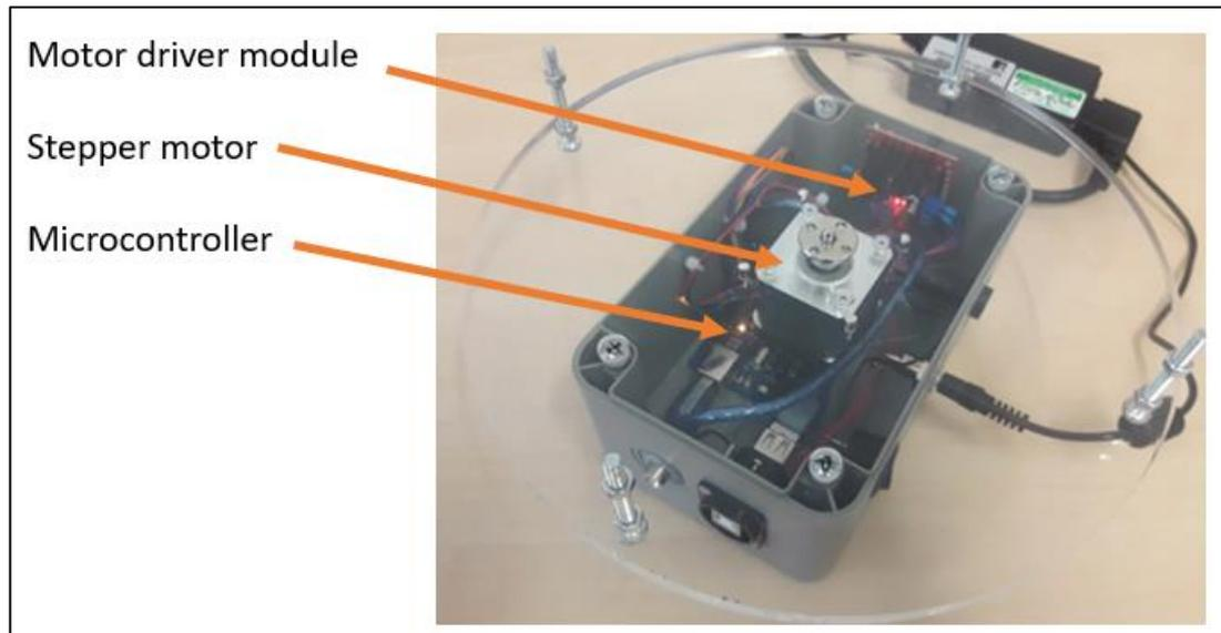
**Figure 6:3:** Assembly of Automated multiplate passive air sampler (AMPAS) component.
