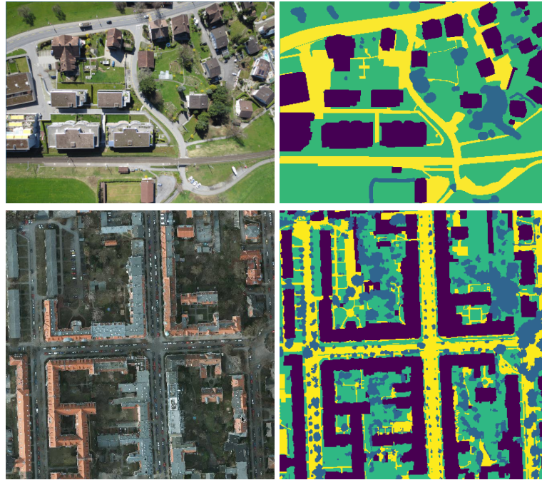
FIGURE 4.3: Top row: Sample snapshots captured by the UAV [2] used for localisation. Bottom row: Sample photo from the CNN training dataset (ISPRS Potsdam [3]). The ground truth for both is composed of four categories: houses, roads, trees and grass
