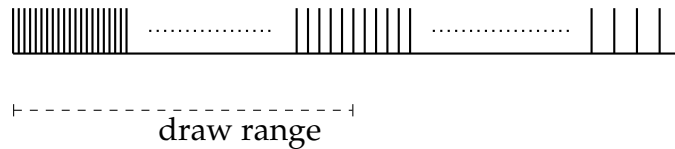
FIGURE 4.12: The cumulative sum of particle weights, notice that it is denser at one edge than the other. Each pin represents an entry, entries at the dense edge are closer match to the measurement (snapshot histogram).
