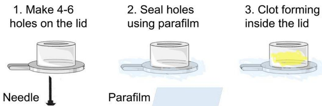
**Figure 2-6.** Graphical representation of SEM sample preparation. Original image of Eppendorf lid was adapted from <https://smart.servier.com>.
