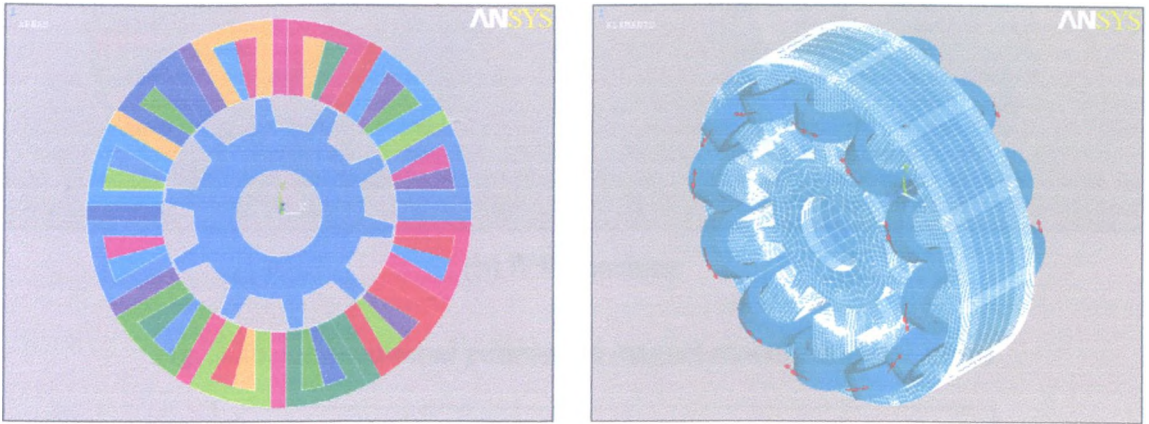
Fig. 2.24 3-D model of flux-switching PM machine ( L_a=25\text{mm} )
