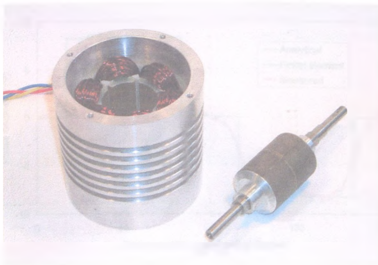
Fig. 4.10. Prototype 4-pole, 6-slot permanent magnet brushless DC machine
