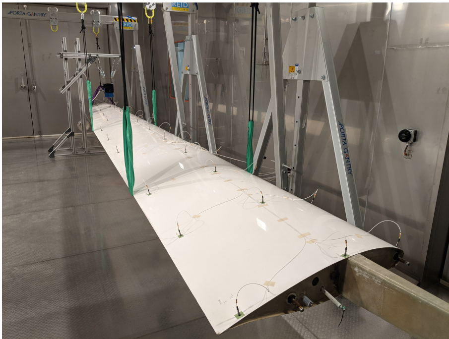
Figure 9.3: Glider wing in temperature-controlled chamber.
