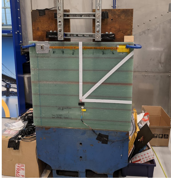
Figure 7.3: Photo of the GFRP plate experiment setup.
