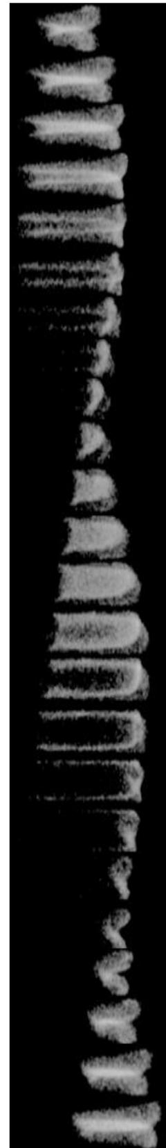
Figure 6.13: Representative images for flame behaviour in different regimes of methane on  $\phi = 1.4, R_H = 0$  flame,  $\phi = 1.5, R_H = 0.4$  flame, and  $\phi = 1.2, R_H = 0.4$  flame. Interval of  $1/2000$  second increments for each frame downwards
