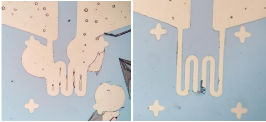
Figure-7.5: Optical microscope image of developed microheater with unremoved Au which causes a short circuit (Left) and burnt out microheater (Right).
