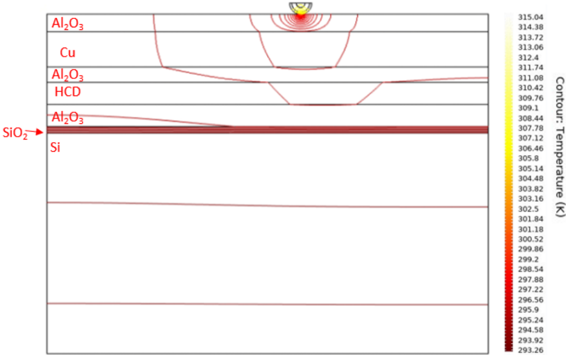
Figure-5.14: Image of COMSOL model of heated tip over multilayer stack showing thermal contours travelling through different material layers.
