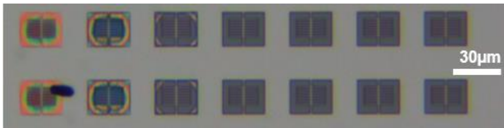
Figure-6.4: Image of ion etching dosing test to determine clearing dosage on large Si fishbones with applied area dosage increasing from the left to right.
