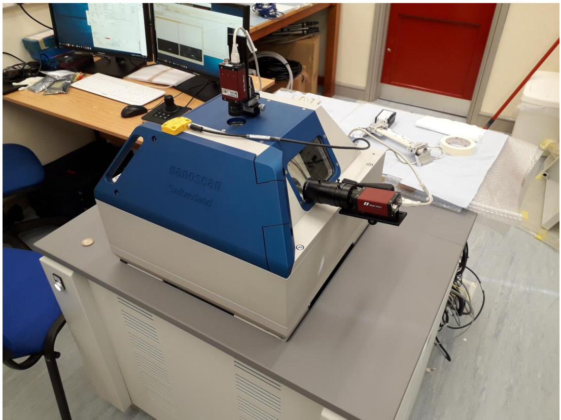
Figure-3.2: Image of sealed chamber of VLS-80 showing externally mounted cameras for positioning the tip.
