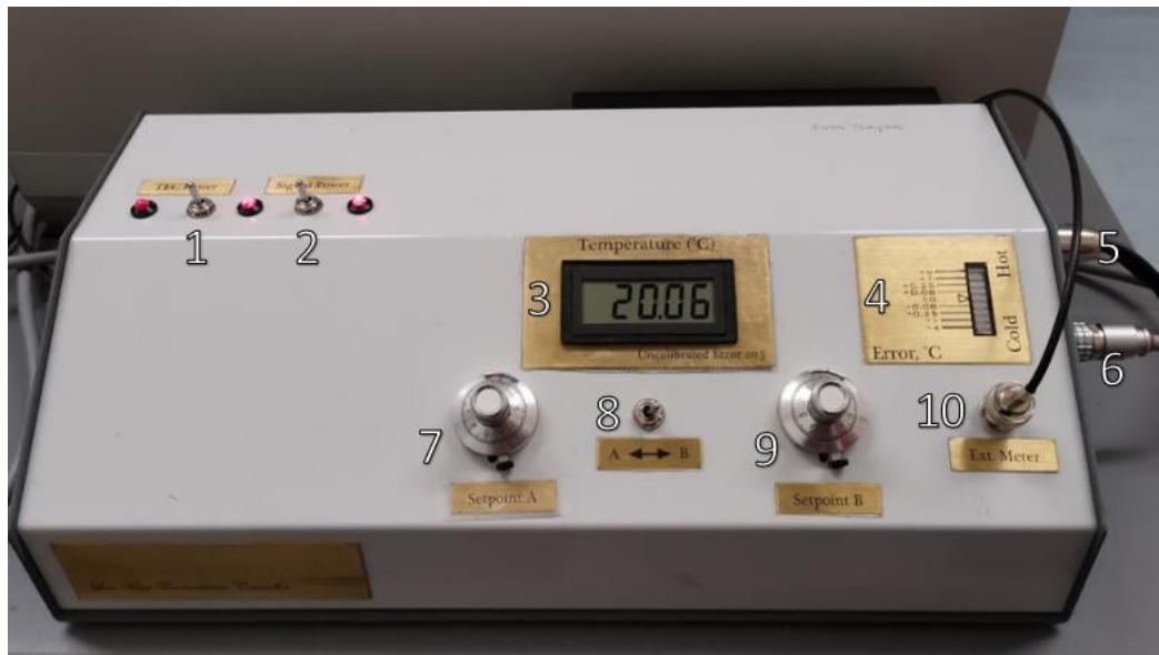
Figure-3.10: Labelled image of the ‘York Low Noise Thermoelectric Control System’. Key: 1. Power Out Switch, 2. Read-out Switch, 3. Temperature Read-out, 4, Error Gauge, 5. Power In Cable, 6. Power Out/Signal In Cable, 7. Temperature Setpoint A Dial, 8. Temperature Setpoint B Dial, 10, Signal Out Cable.
