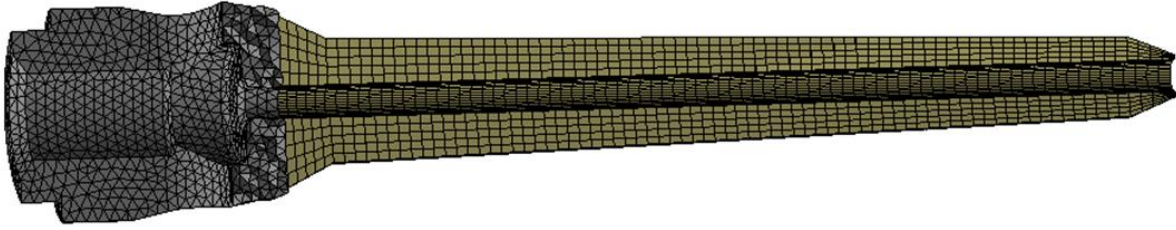
Figure 4.2 – Mid-section view of the mesh of the screw. The head of the screw is meshed with tetrahedral elements, while the remaining part is meshed with a structured hexahedral mesh.
