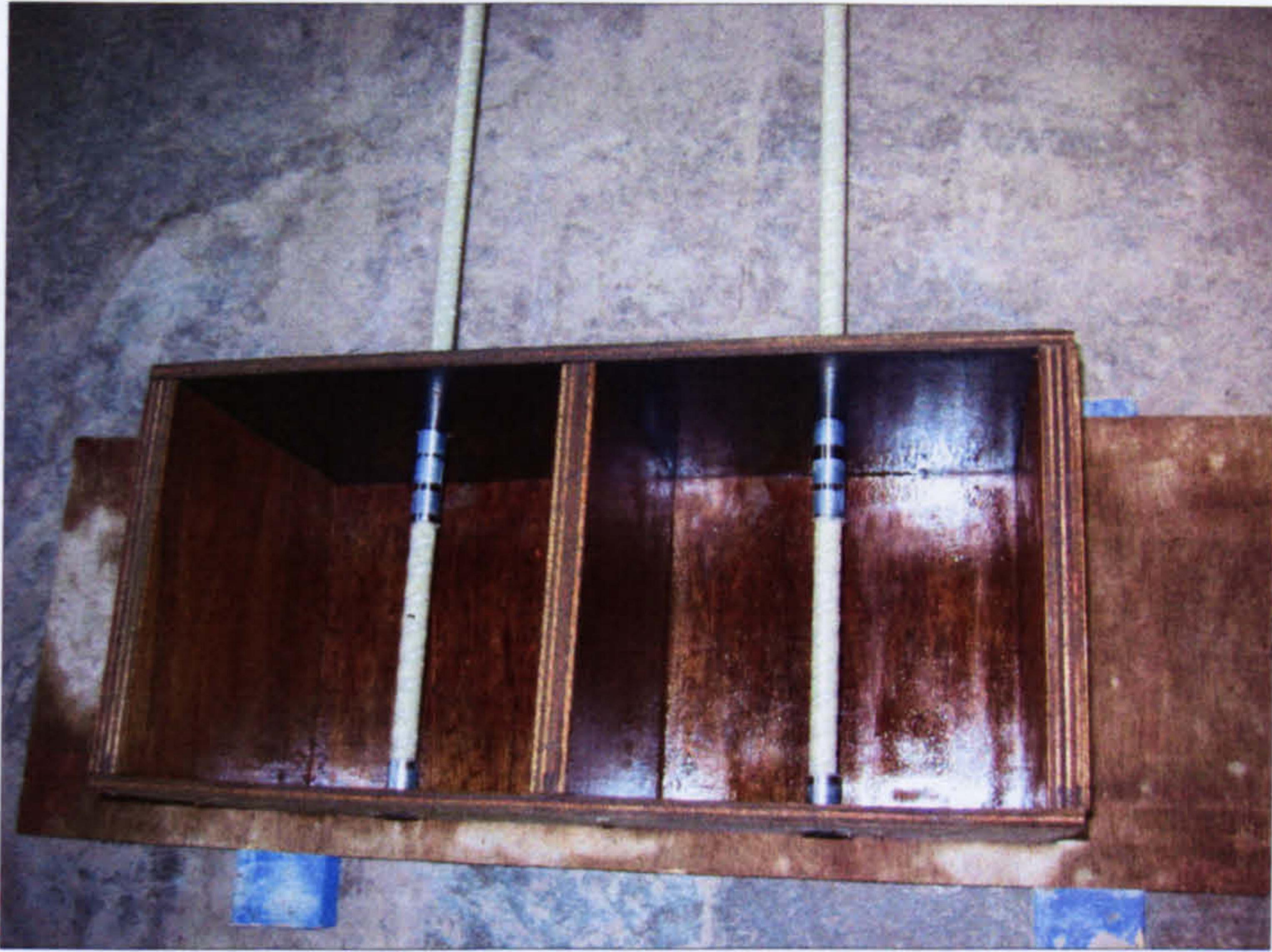
Fig. 5-4 Prepared moulds for pull-out test just before casting of concrete
