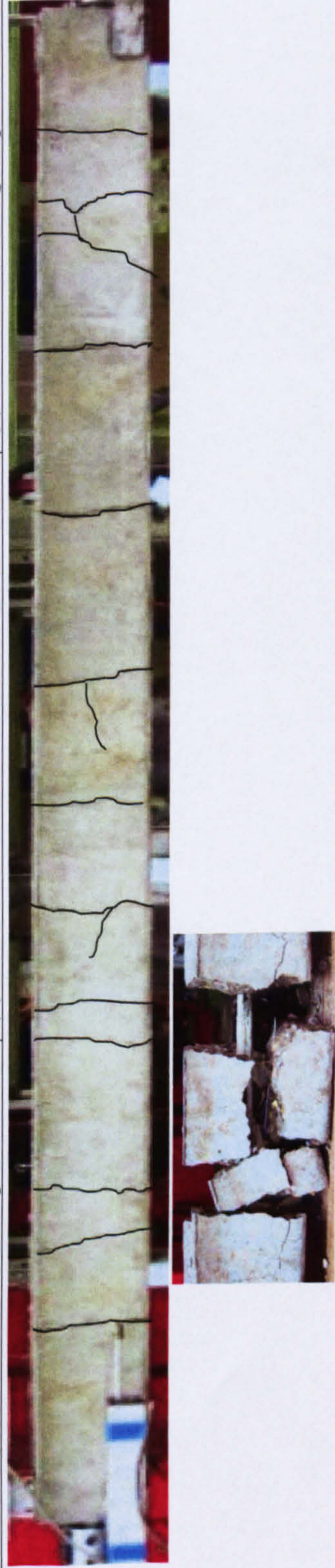
(a) Crack pattern of tested specimen & final failure of the bar
