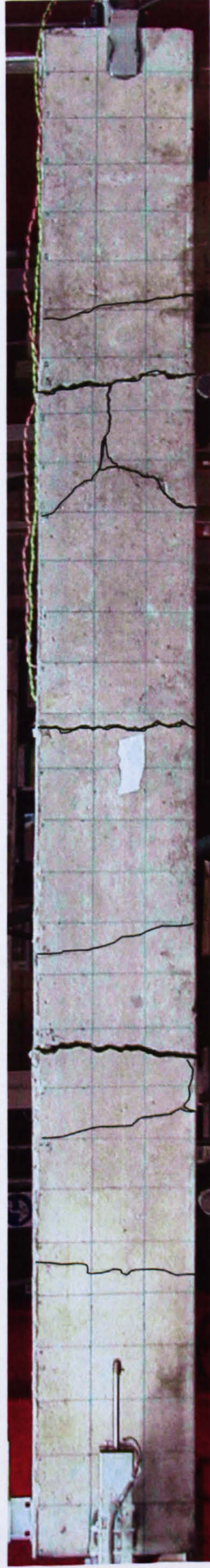
(a) Crack pattern of tested specimen
