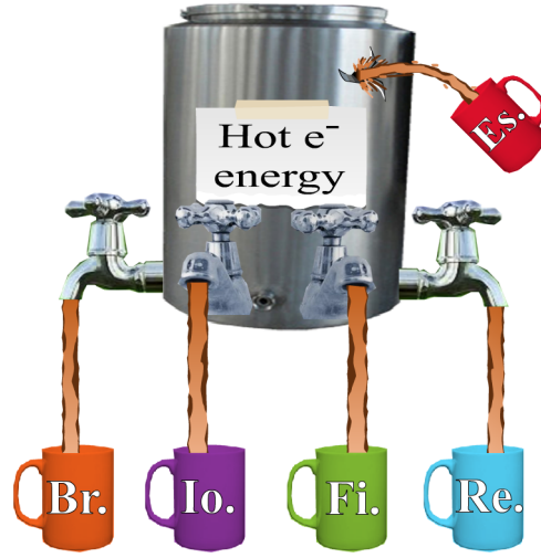
Figure 7.1: Visual representation of different processes simultaneously competing for the same electron energy. Labelled processes include bremsstrahlung (Br.), ionisation energy loss (Io.), resistive field losses (Fi.), reflux losses in the sheath fields (Re.) and escaping electron energy (Es.).
