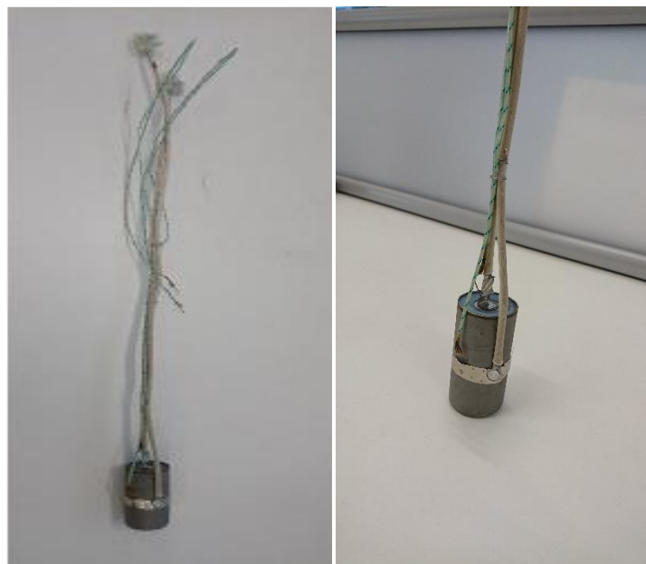
Figure 3-2: Cell with connections showing the connection points of the electrodes and type k thermocouples
