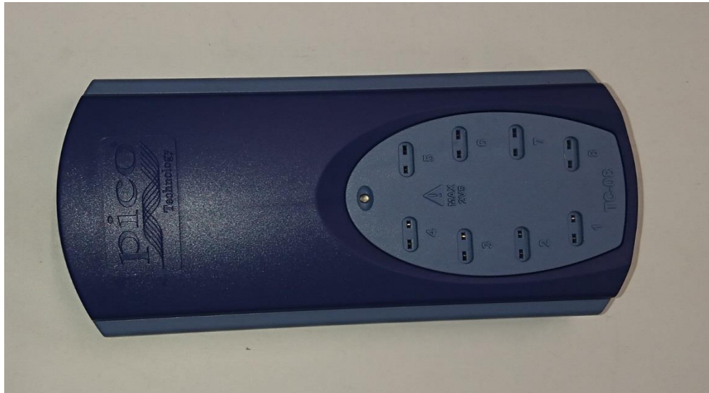
Figure 3-10: Pico TC-08 Datalogger
