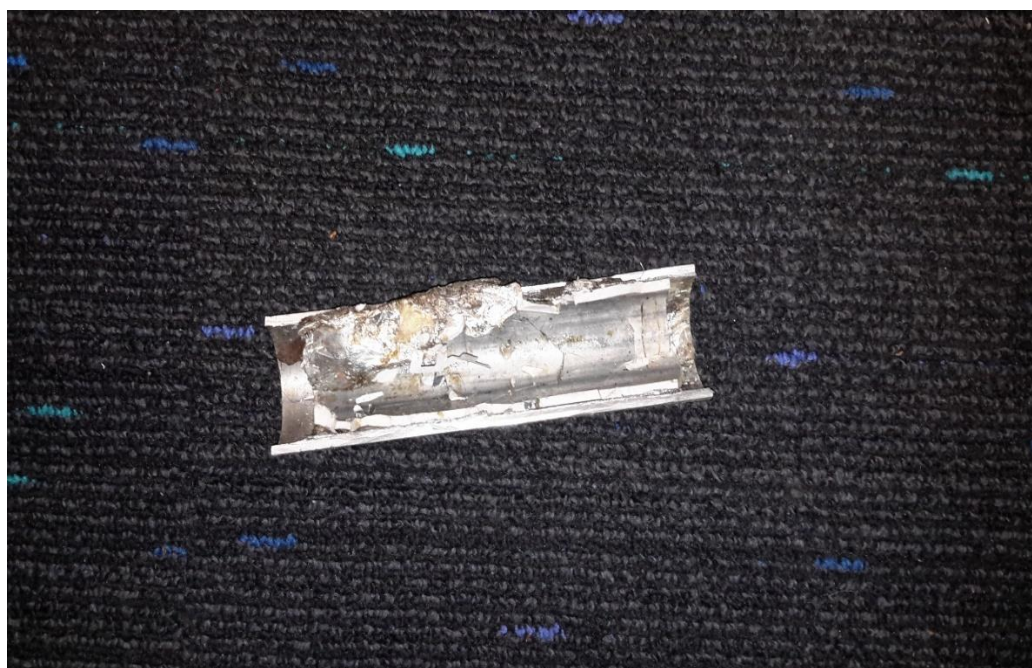
Figure 4-1: Cracked mullite alumina ceramic tube
