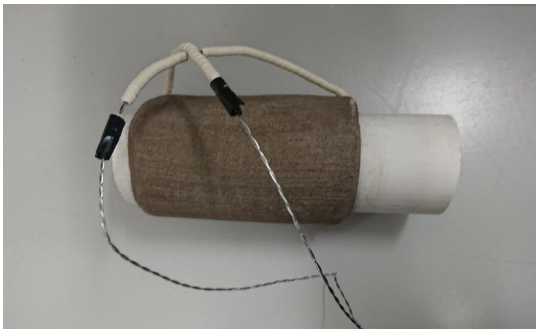
Figure 3-7: Heating element of the furnace tube
