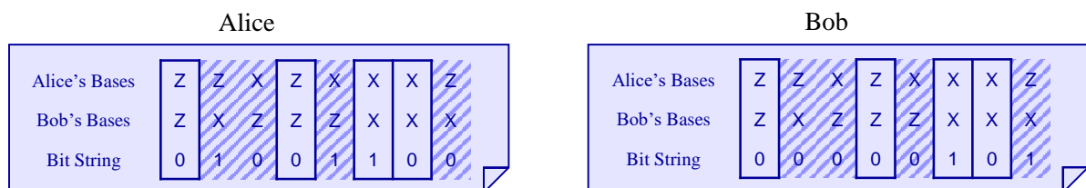
Figure 1.3: Depiction of basis reconciliation performed by Alice and Bob to distill the key from the shared bit string in the BB84 protocol. If Alice and Bob use the same basis to prepare and measure the quantum state, they keep the bit value. If Alice and Bob use different bases to prepare and measure the quantum state, they discard the bit value (crossed out).
