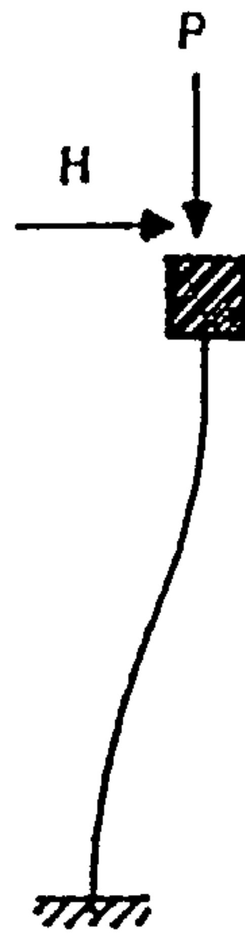
Figure 9.22.a: Column with perfect rotational end restraints
