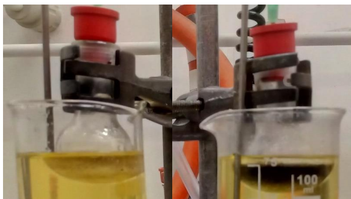
Figure 3.3.1: Left: Suzuki-Miyaura reaction mixture in ChCl/U after stirring for 10 minutes at 100 °C. Right: Suzuki-Miyaura reaction mixture in ChCl/G after stirring for 10 minutes at 100 °C
