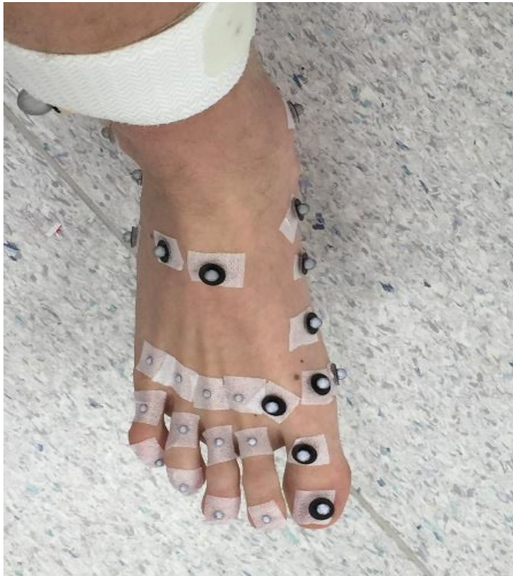
Figure 19 Motion capture marker set up of the foot for the GM foot model.
