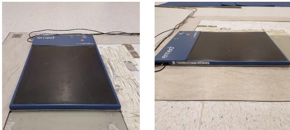
Figure 21 Image of pressure platform set up in the laboratory used to collect pressure data from patients that could be used in the 26-segmentfoot model
