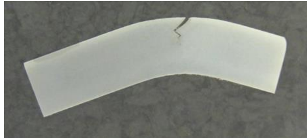
Figure 2-23: left: S960 steel, 3 point-bending with 13mm stroke [14].
