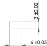
Figure 4-6: Drawing for the production of 3mm thickness bend test specimen design for the Deben 5mm diameter tooling.
