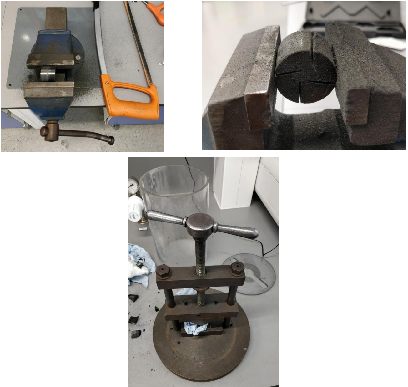
Figure 3-6: Method of breaking samples out of mountings, top left; clamping before sawing with hand saws, top right; specimen with cuts from sawing to weaken the mounting, bottom; mounted specimen wrapped in cotton wool and paper towels to protect the surface and retain mounting fragments in the mounting breaking clamp.
