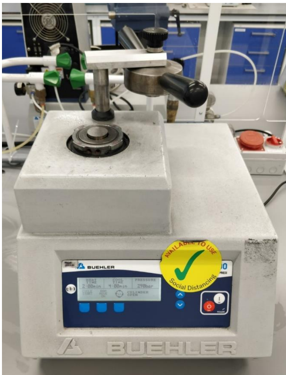
Figure 3-5: Buehler SimpliMet 1000 v3 automated mounting press
