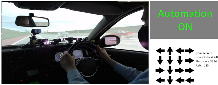
Figure 30: Cab interior of the UoLDS with presented motorway scenario (left). The left side of the cluster was presenting the speedometer while the right side was used to display ADS status. When blank (as in the left picture) HAD was off. When drivers were in HAD, the cluster displayed the picture on the top-right corner. On the bottom-right corner, the presented arrows task displayed on a touch-screen tablet placed on the left side of the driver.
