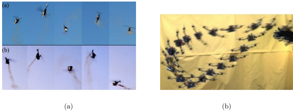
Figure 2.11. Examples of UAV projects that have good manoeuvrability or recoverability based on RL algorithms where (a) shows the manoeuvres performed on a Stanford helicopter through inverse RL, reprinted from [114] and (b) shows the hand throw recovery implemented on a ETH quadcopter through RL, reprinted from [36].
