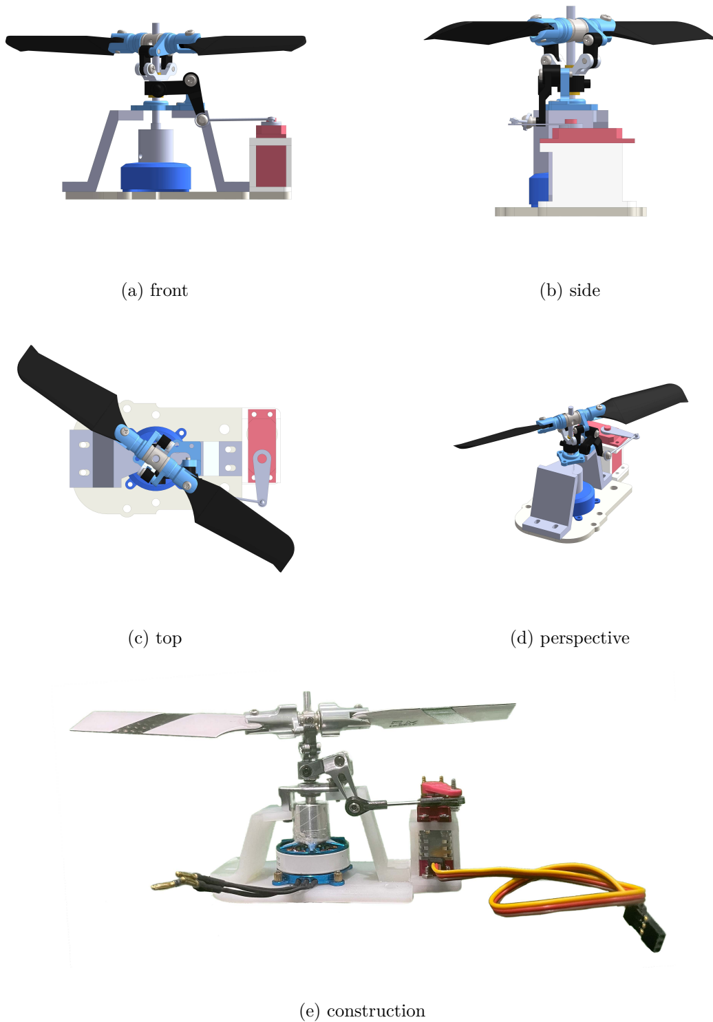
Figure A.1. VPP actuator design. (a)-(d) show the mechanical design from different perspectives and (e) shows the actual construction.
