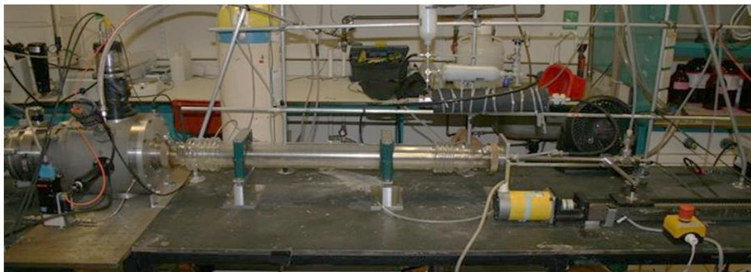
**Figure 2.4.** Aerosol flow tube setup showing connection to the FAGE cell of the right. Sliding injector is shown on the left.
