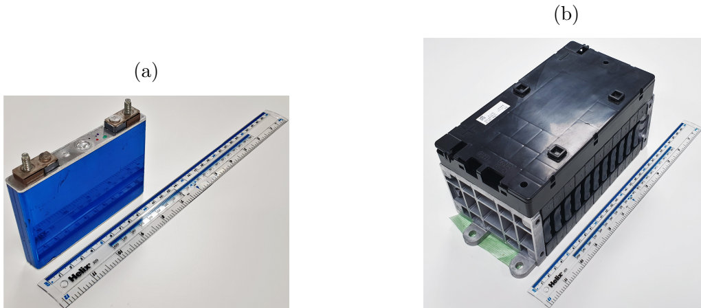
Figure 3.1: Yuasa LIM5H cell (a), removed from LIM5H Module (b).
