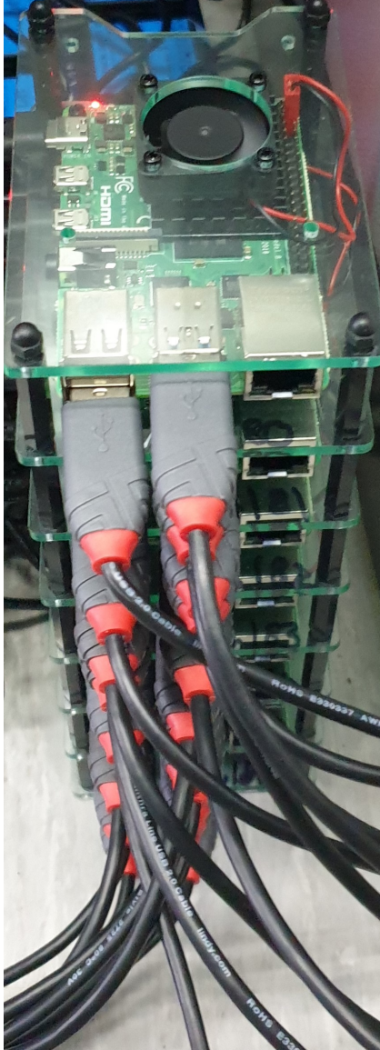
Figure 3.12: (a) Raspberry Pi 4 cluster and, (b) USBtin Device, used together to monitor cell voltage at WESS.
