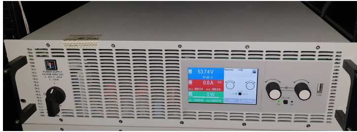
Figure 3.7: EA-PSB 9080-240 power supply used for cycling modules below 80V, this is identical in appearance to the EA PSB 9750-60 which is used for cycling modules up to 750V.
