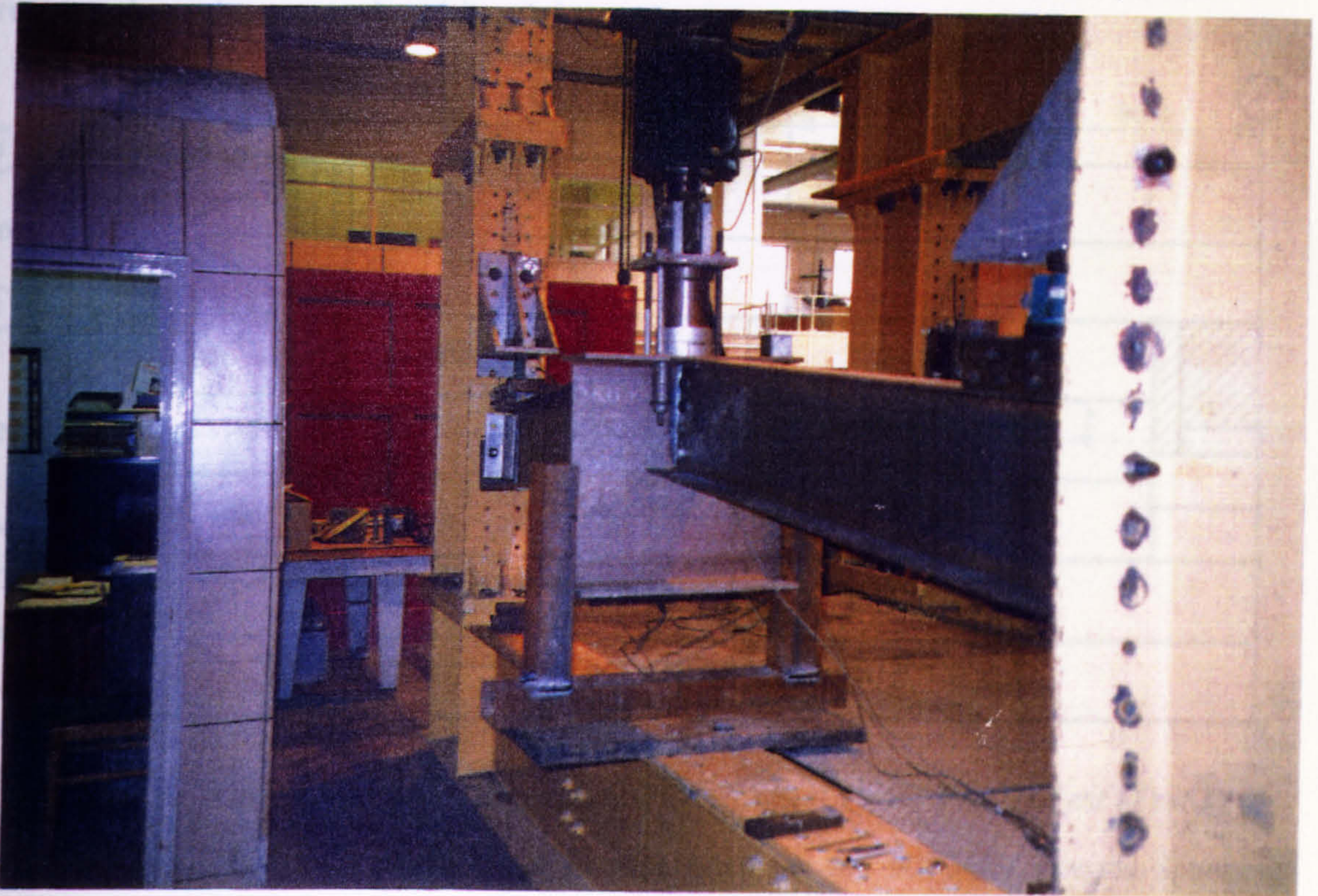
Figure 7.5. Ambient-Temperature Cruciform Beam-to-Beam Test Arrangement
