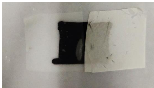
Figure 29. Opacity changes of PCL RES with air plasma treatment (left) and with no plasma treatment (right) after 6 hours of being incubated in PBS at 37 °C, 5 % CO 2 .
