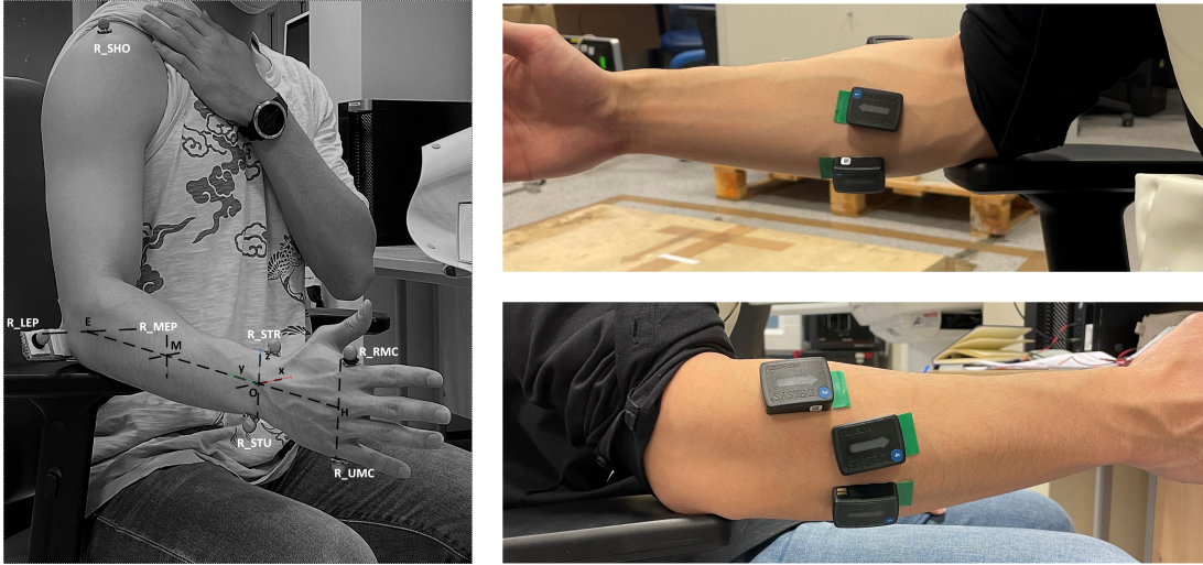
Figure 6.1: The placement of electrodes (right) and markers position of the right limb (left), along with the corresponding coordinate system. Markers on each limb are attached symmetrically.
