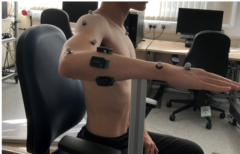
Figure 3.5: Experimental setup 16 reflective markers are attached on subject's right upper limb. Electrodes are placed on five primary muscles of wrist joint including FCR, FCU, ECU, ECRL and ECRB.
