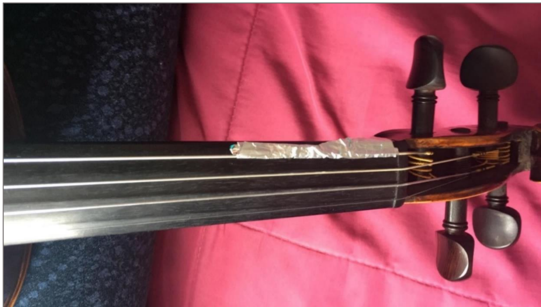
Figure 56. Photograph of the violin preparation by wrapping 4cm of string IV (scordatura E3) with aluminium foil. 169
