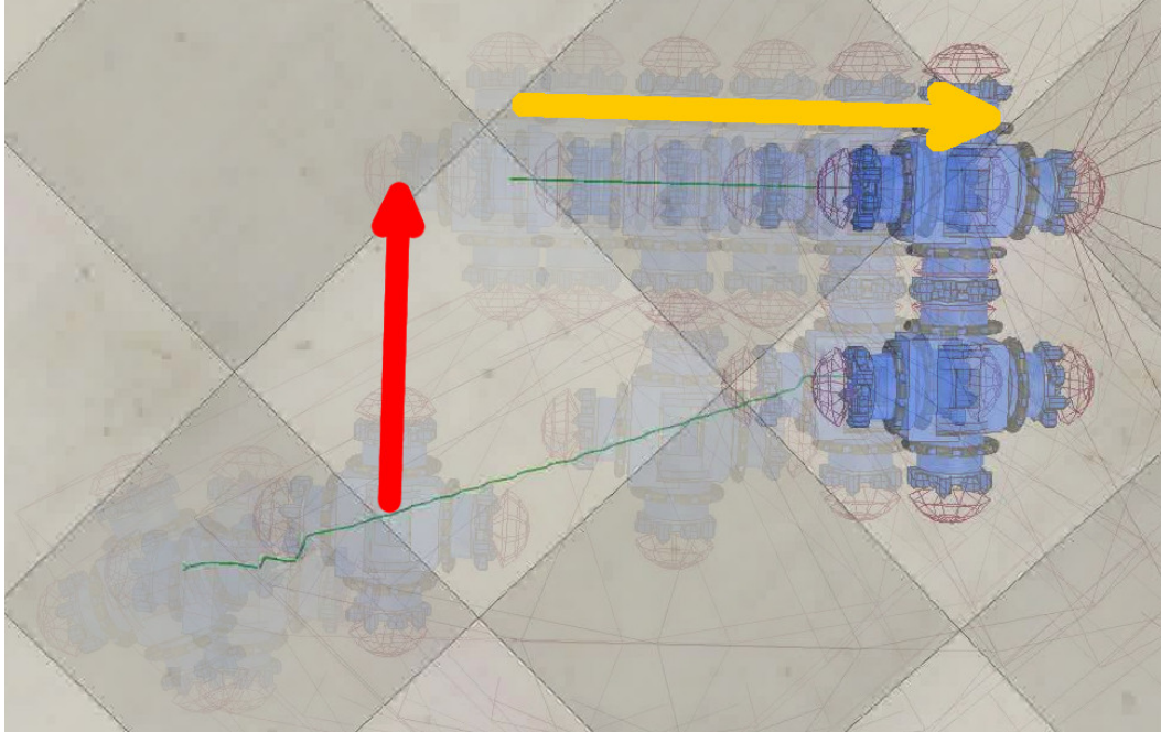
Fig. 4.18: To fix the misalignment in the last few centimetres the approaching robot makes all motions relative to the, moving, reference frame of the recruiter. In the recruiter's reference frame the final docking motions are straight inwards (red arrow) whereas in the reference frame of a ground observer the final motions are angled (green ground track). The yellow arrow shows the recruiter's motion. For a non-moving seed the mathematics used in the controller for this reference frame based docking simplifies to exactly that used in stationary seed docking.
