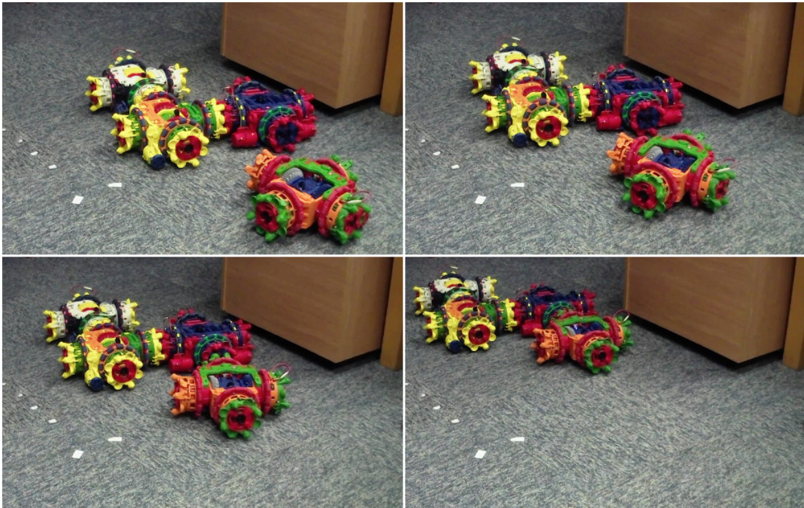
Fig. 6.22: A robot is placed at a random orientation within IR communication range of a docking port and matches compass alignment and position to dock.
