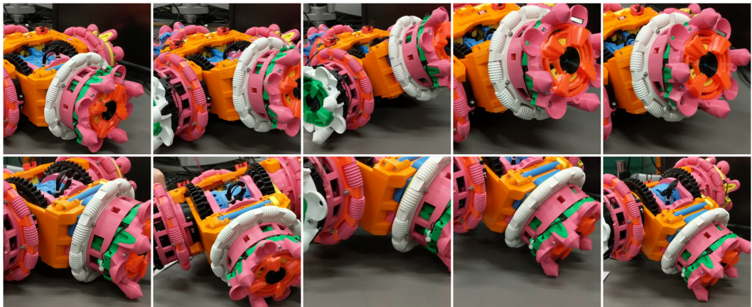
Fig. 5.17: Testing of the hinge system with a partly assembled robot and temporary external driver circuitry. The upper series of images shows the hinge elevating Port 4's pitch to 45^\circ then rolling Port 4 clockwise. The lower series shows the robot raising itself up by pitching the hinge downwards, even while lifting the weight of the robot, currents did not rise above a 240 mA peak. A video of the test's highlights is available at [212] and in the supplementary material (Early_hinge_test.mp4).
