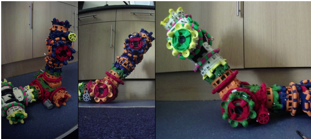
Fig. 5.35: The new hinge design in use, pitching and rolling other robots. The robot on the ground behind the actuating robot serves as a counterbalance for the lifted module.
