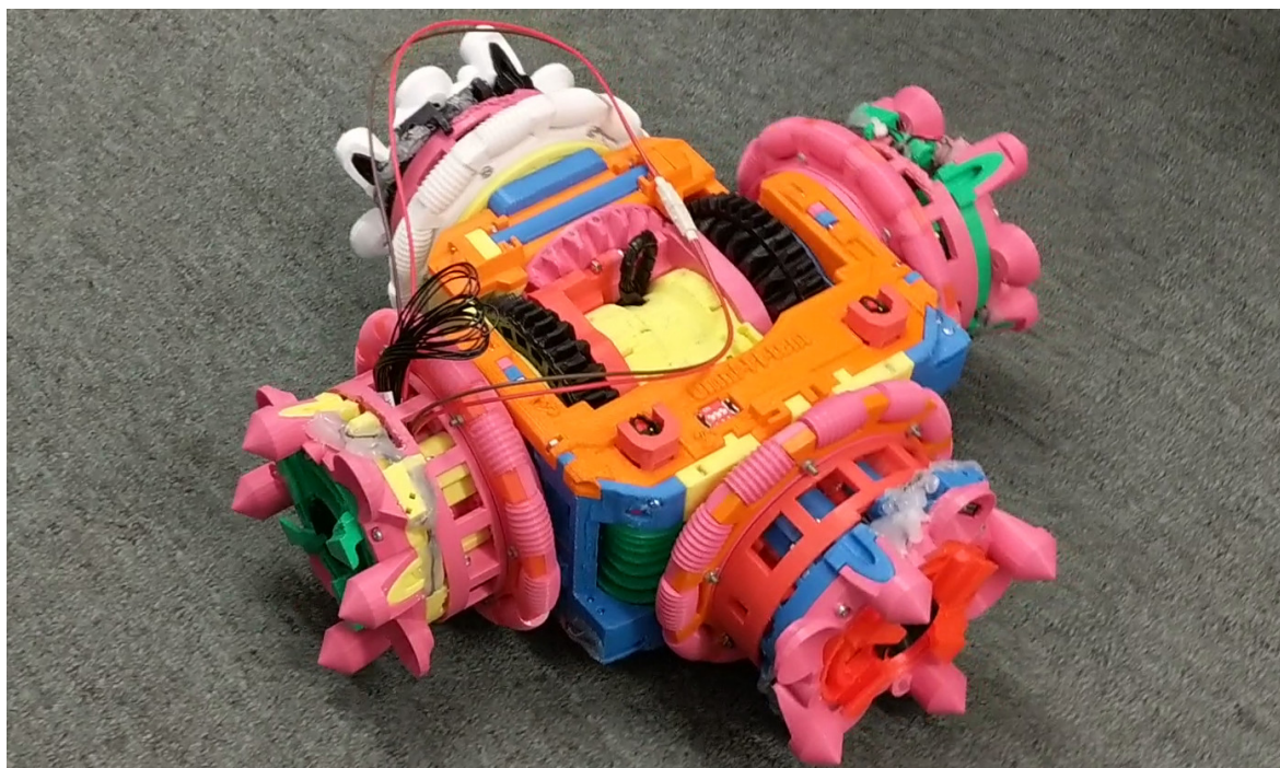
Fig. 3.13: The first prototype module, viewed from above and behind. Colours of the component parts reflect which material was in the printer at the time an element was designed or revised, this has a side-effect of making the separate elements of the design and joins between them easily identifiable.
