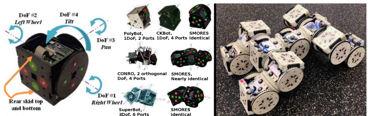
Fig. 2.6: A SMORES robot with the degrees of freedom marked (left), is shown alongside a comparison to other modular platforms (centre) showing how one or a small number of SMORES modules can represent the geometry of those designs and copy their degrees of freedom. Also shown is a mobile multi-robot structure using the slightly later SMORES-EP module design. Images from the papers [35] and [5].
