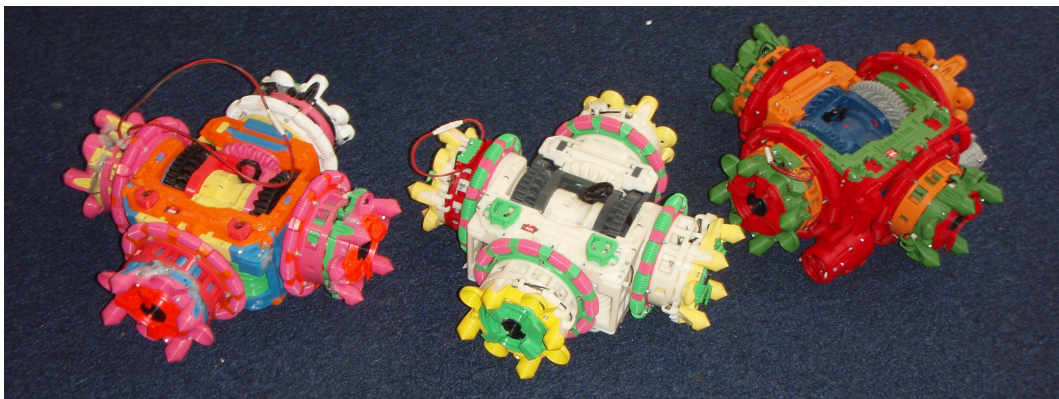
Fig. 5.41: The first prototype (left), the second prototype (centre) before upgrading with the new hinge components, and the first production module (right) after upgrading with new hinge and wheel parts. The changes between the versions improved subsystem effectiveness but did not not change the intended functionalities, hence all versions have a broadly similar outward appearance.
