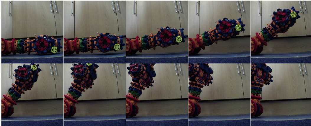
Fig. 5.36: Time series photographs showing the new hinge elevating to pitch and then roll another robot. A video is available at [214] and in the supplementary material (Hinge_actuation_tests.mp4)
