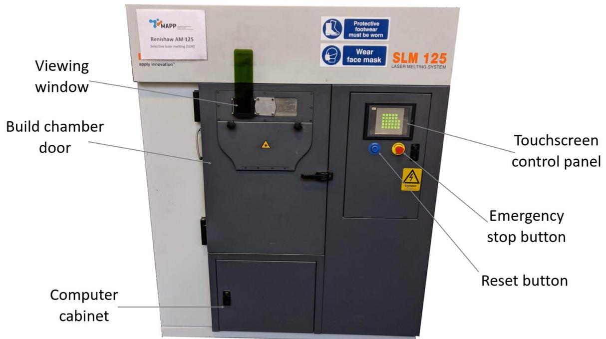
Figure 3.5. Renishaw SLM 125's outer view.
