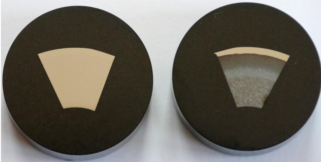
Figure 3.5: Polished (l) and etched (r) R260 grade SUROS with MSS laser clad coating samples
