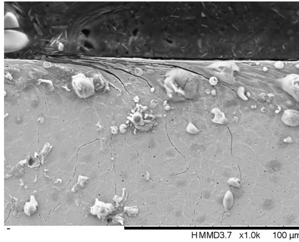
(c) Strain accumulation in MSS laser clad coating after 10,000 cycles. (Sample contaminated however the angle of deformation could still be gathered.)
