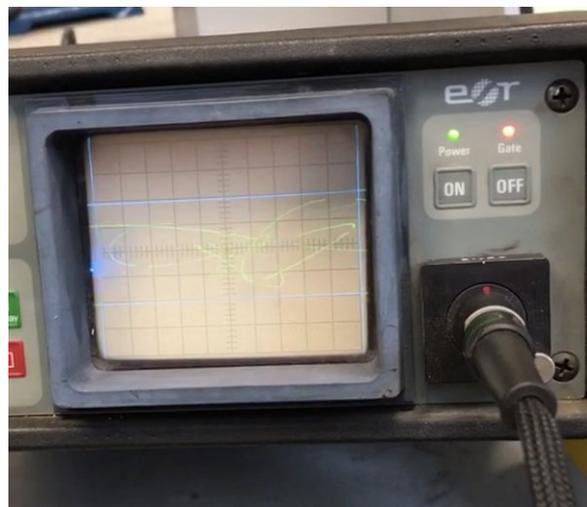
Figure 4.7: Eddy current detector signal over the untested repair disc, gates triggered at each joint between parent rail and repair.
