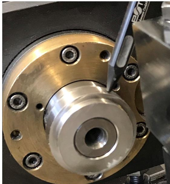
Figure 4.5: Position of KD21 Rohmann GmbH differential eddy current probe positioned over the R1 45 calibration disc.
