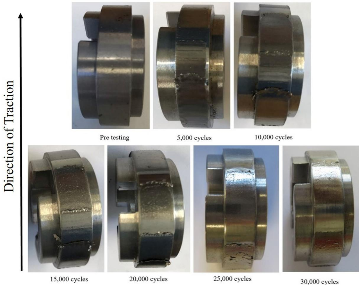
Figure 4.24: Visual observation of the progression of surface evolution on the repair disc at regular intervals in the unlubricated test. Material flow can be seen at the interface between the parent rail and repair sites.
