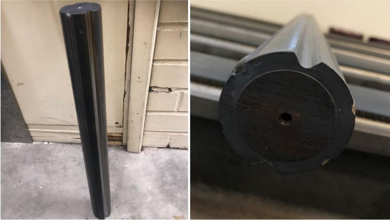
Figure 4.1: Photograph of the repair bar during the manufacturing process showing the wire eroded slots for the laser clad repairs.
