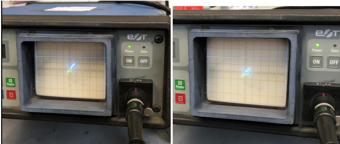
(a) Standard R1 45 calibration disc of R260 grade rail steel. (b) R260 grade rail steel rail disc with full MSS laser clad surface.
