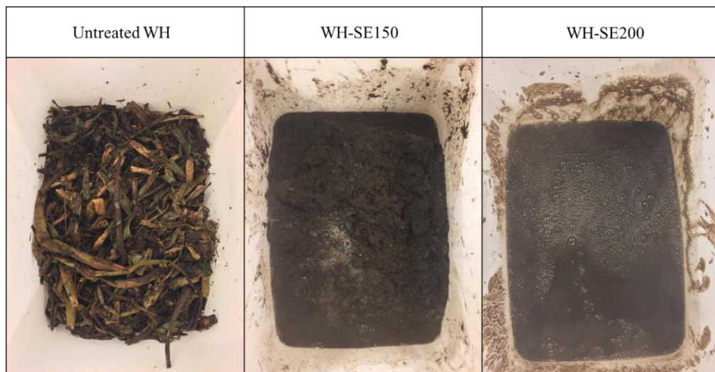
Figure 7.6. Physical appearance of WH following steam explosion at 150°C and 200°C.
