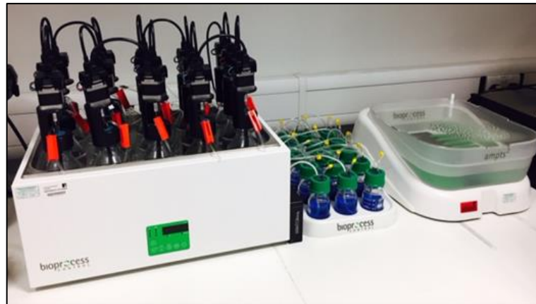
Figure 3.3. Automatic Methane Potential Test System II.
