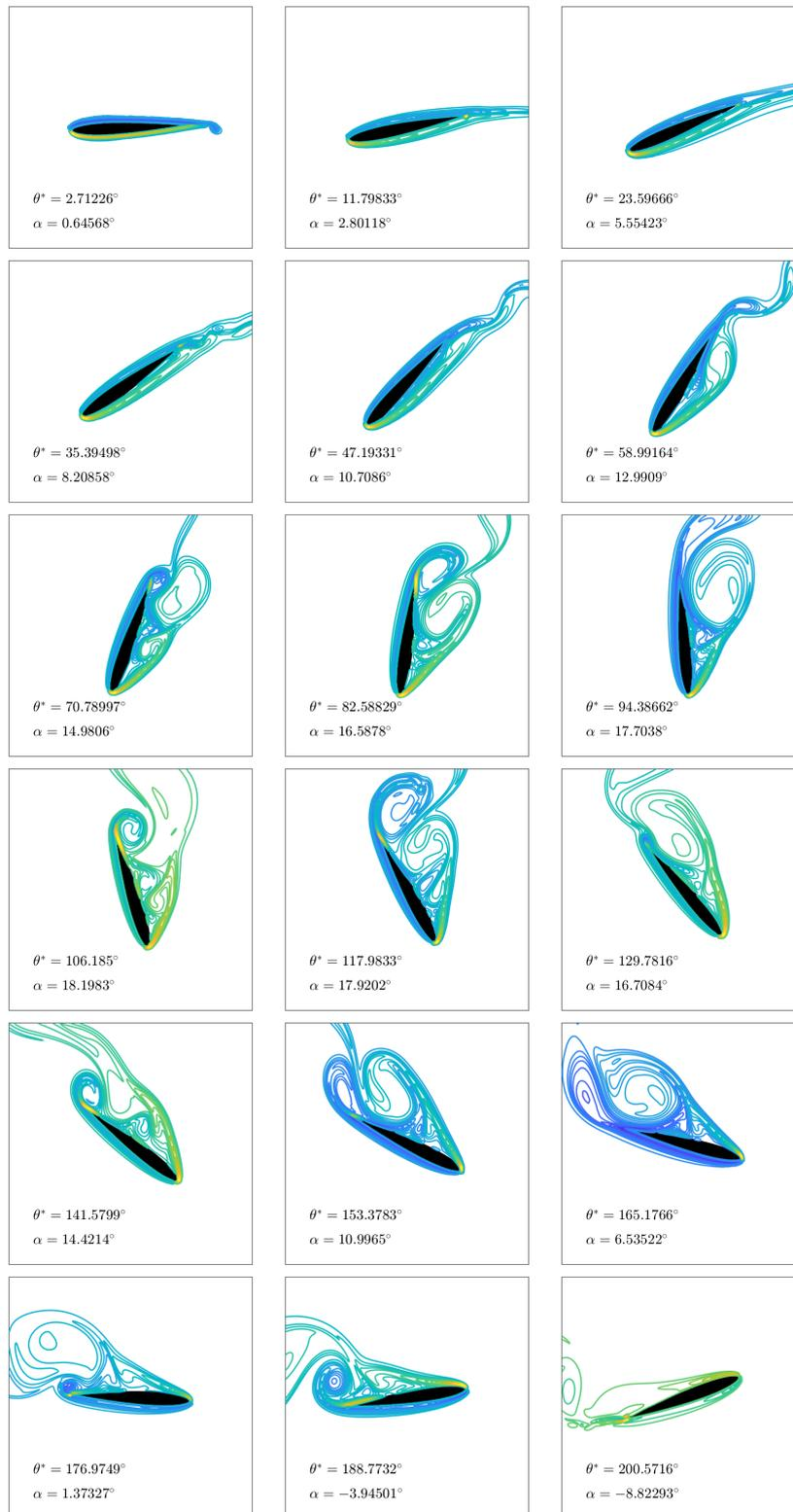
FIGURE 7.14: The vorticity contour depicting the full sequence of the aerofoil motion in the upstream part of the VAWT cycle.  $\theta^*$  is the shifted azimuthal angle.
