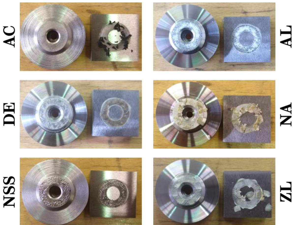
Figure 5.37. Post-test Specimens with Other Particles applied in Wet Conditions.
