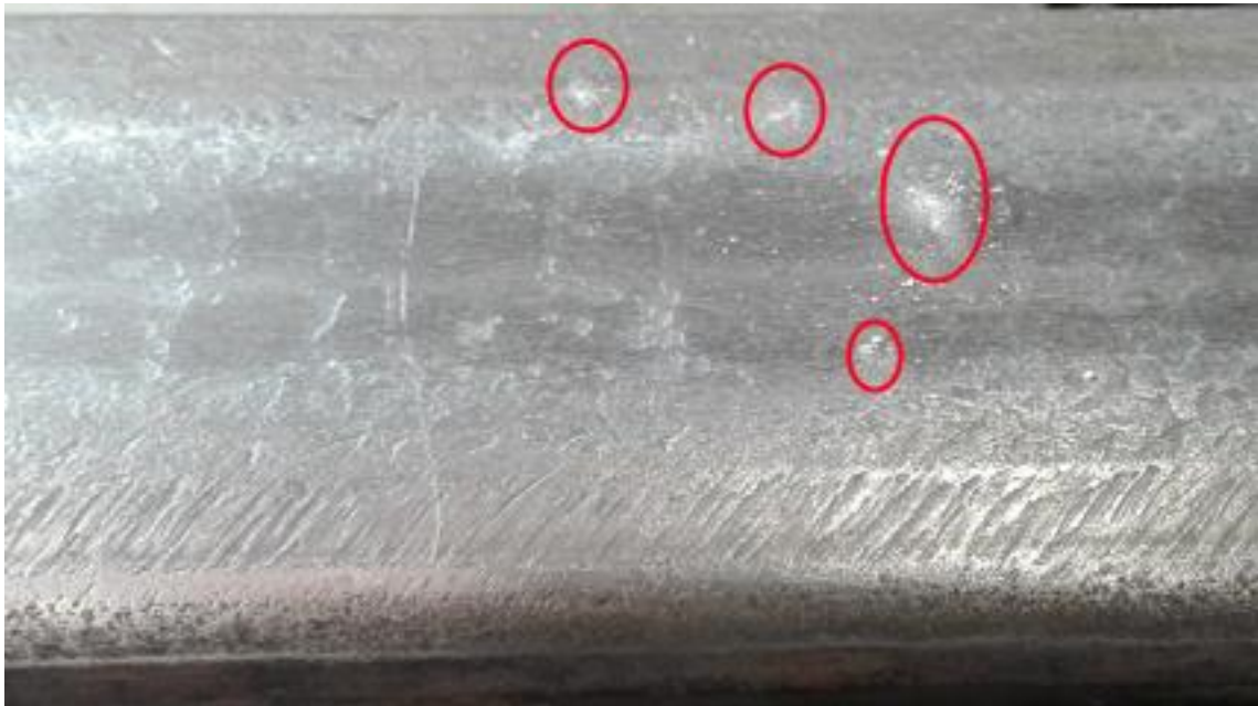
Figure 6.3. Rail Head Post-Wheel Pass over a Single LB Particle with Remaining Material Encircled.
