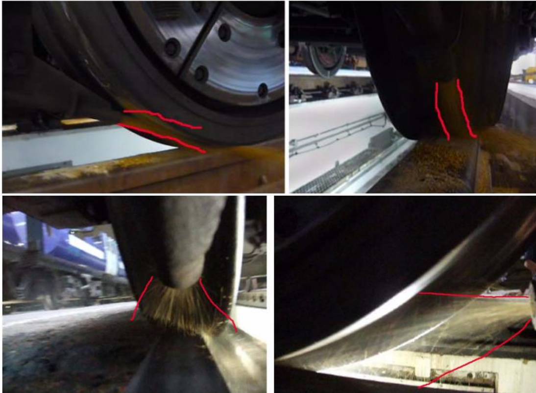
Figure 3.25. (Top) Narrow Discharge Pattern vs (Bottom) Wide Discharge Pattern [17].
