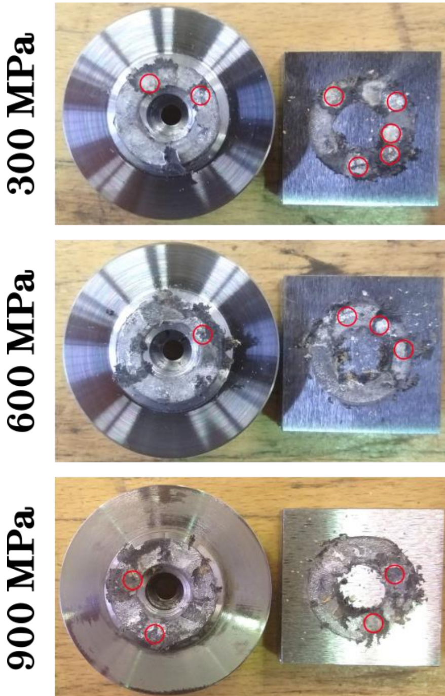
Figure 5.74. Post-test Specimens with LB applied in Leaf Contaminated Conditions with Varying Contact Pressure.
