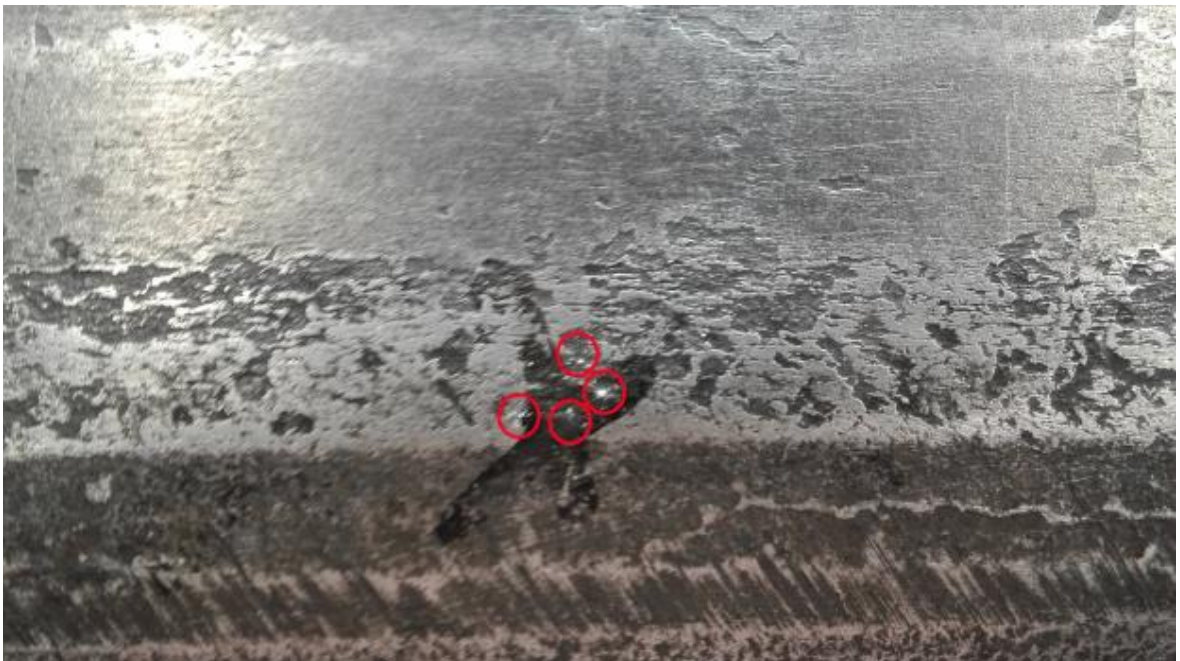
Figure 6.7. Rail Head Post-Wheel Pass over a Single DY Particle.
