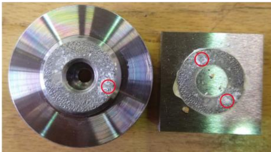
Figure 5.69. Post-test Specimens with LB applied in Wet Conditions with Varying Contact Pressure with Remaining Material encircled.
