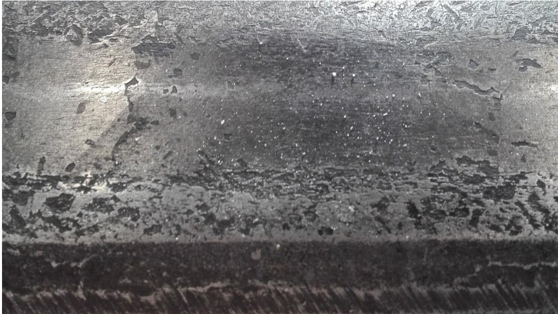
Figure 6.11. Rail Head Post-Wheel Pass over Multiple CE Particles.
