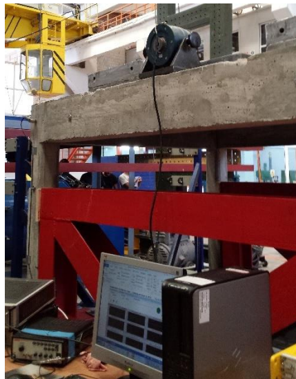
Figure 4.12: Vibration generator fixated on top of the building to determine natural frequencies
