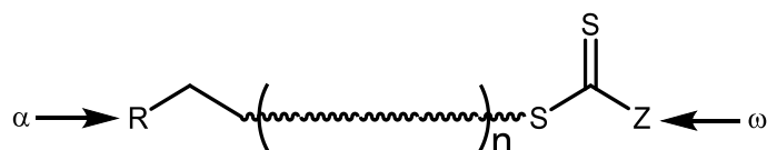
Figure 2.8- The location of the polymer in RAFT polymerisation, showing the \alpha and \omega ends
