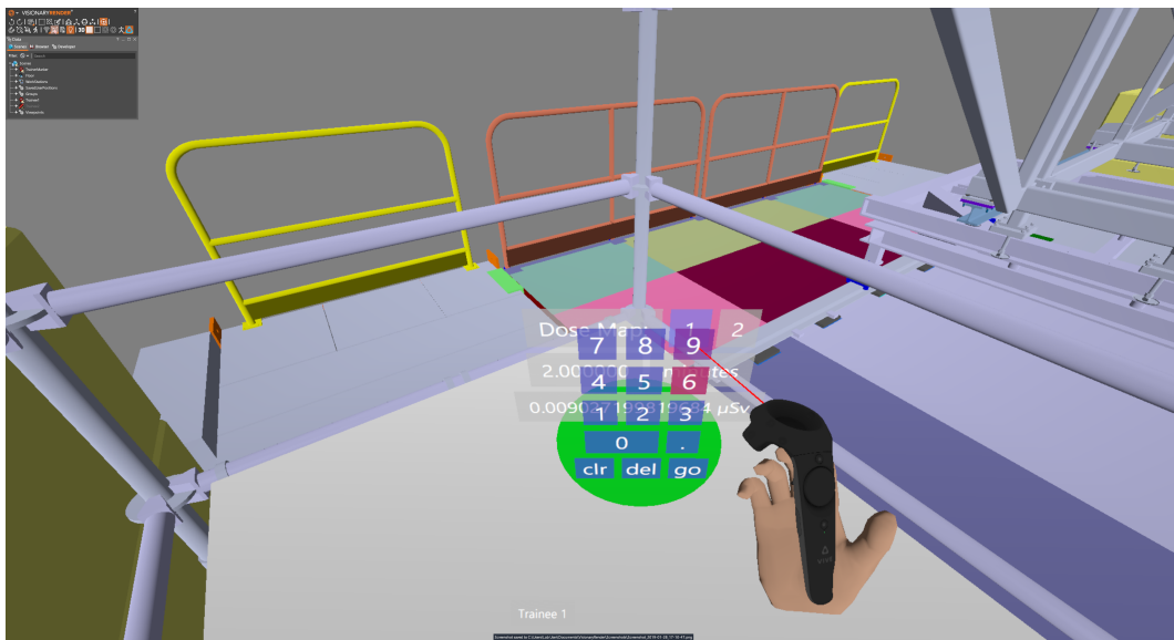
Figure 36: Working inside the VR. A guidance point being modified by a worker wearing a VR headset inside the ATLAS Mockup platform. The hand controller is visible, and the worker is changing the time estimate for the task associated with this guidance point. Once the input is confirmed, the guidance point will recalculate the dose estimate using the new time estimate. The worker HUD is collapsed out of the way at the bottom of the image.
