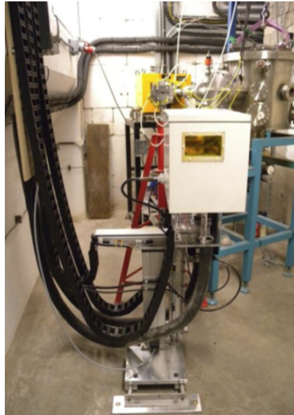
(a) Photo of the Cartesian robot system with radiation box.
