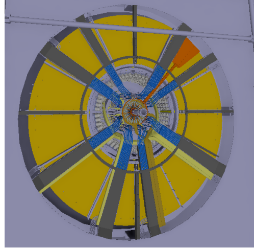
(b) ID with the Endplate nose and Beampipe support removed
