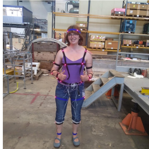
(b) The author wearing the LEDs to calibrate the system and test for occlusions. Velcro strips were used to attach the LEDs to the body.
