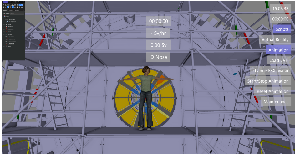
(b) A technician on the scaffolding and ATLAS Endplate in the VR Intervention Planning Platform
