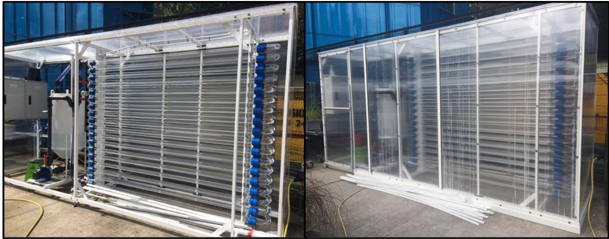
Figure 4.1: 300 L Phycoflow™ unit set up with and without the polycarbonate casing attached.
