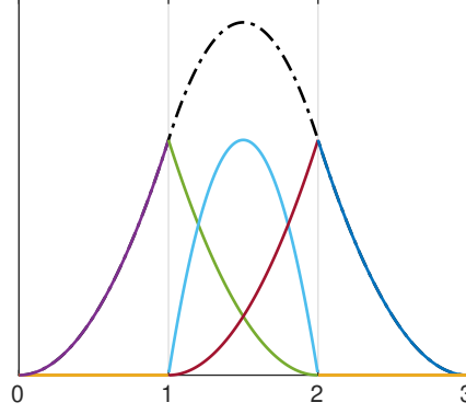
Figure 2.5: Example of Bézier extraction of the dotted B-spline into Bernstein polynomials.
