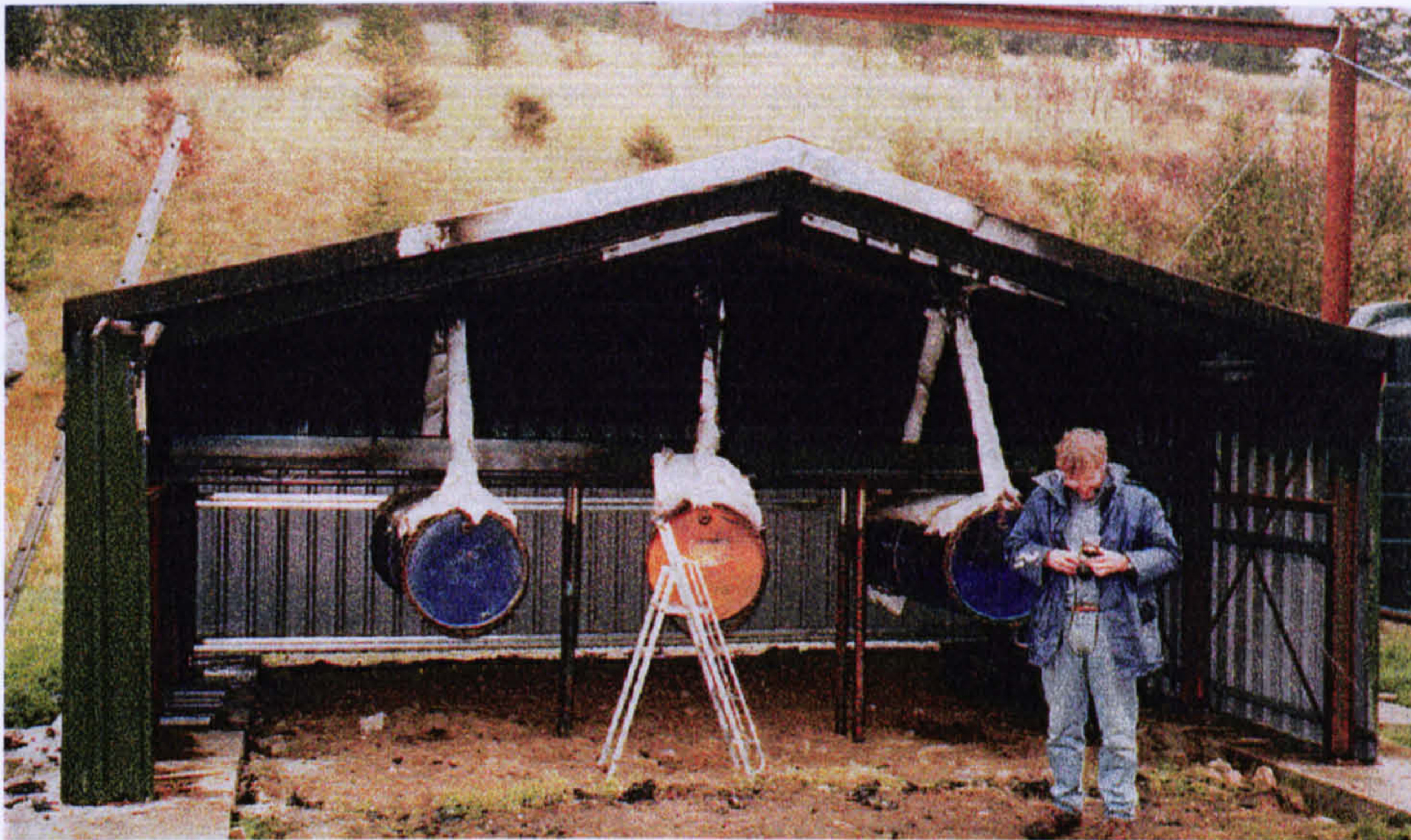
Figure 4.3 The Loading system for the portal frame
