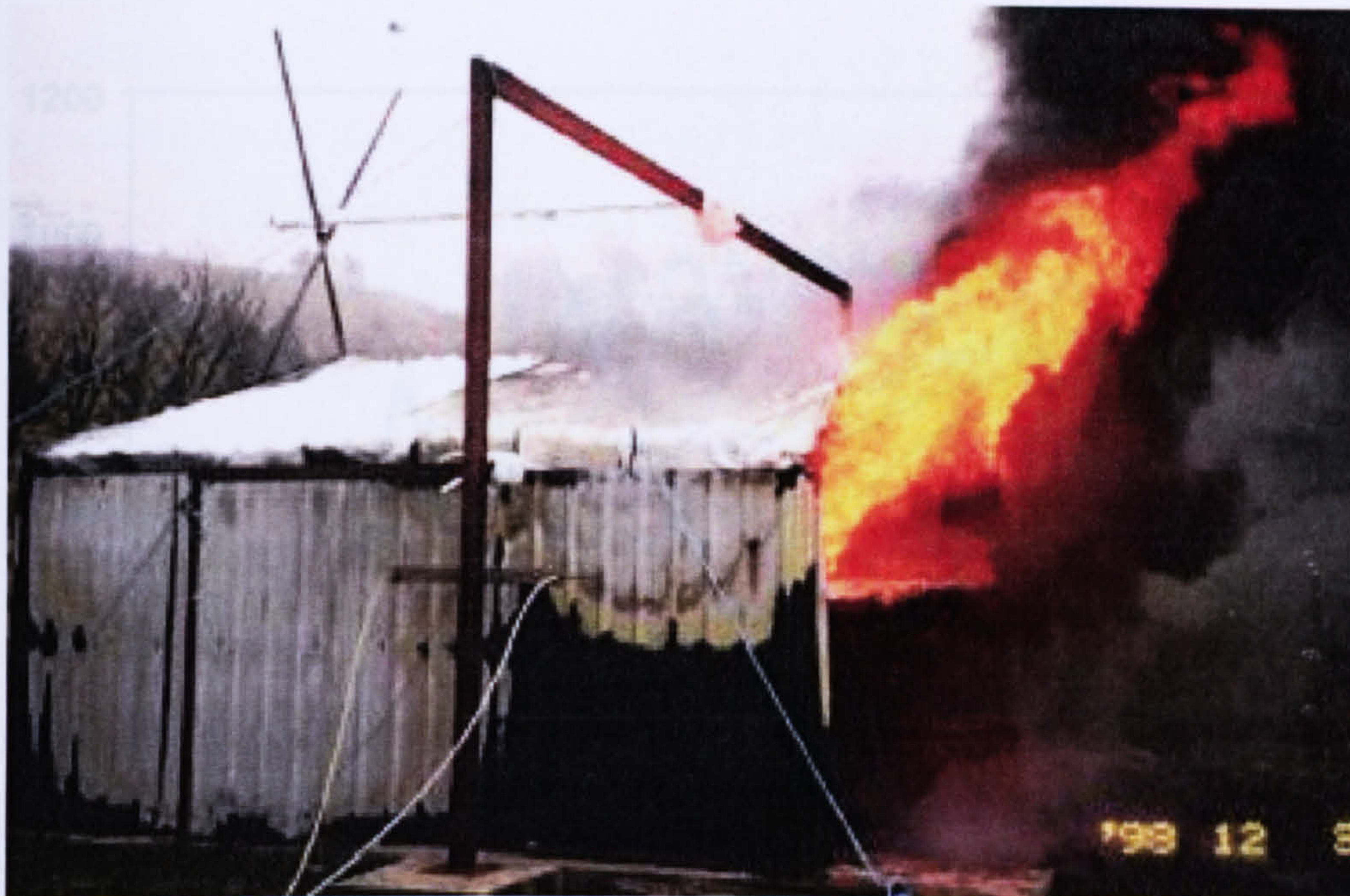
Figure 4.24 Snap-through failure during the third fire test
