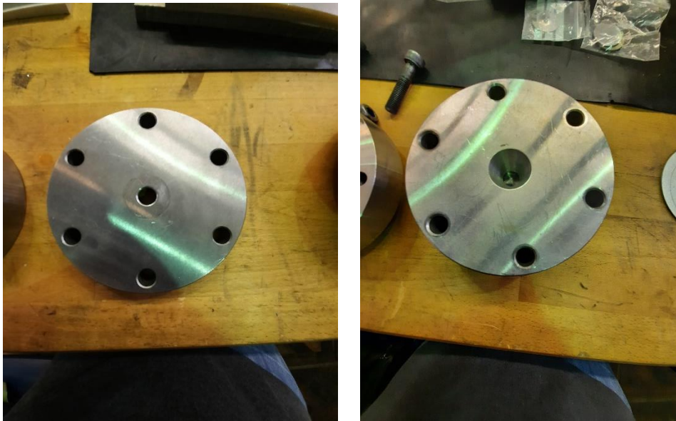
Fig. III. 1 Top and bottom views of top die.
