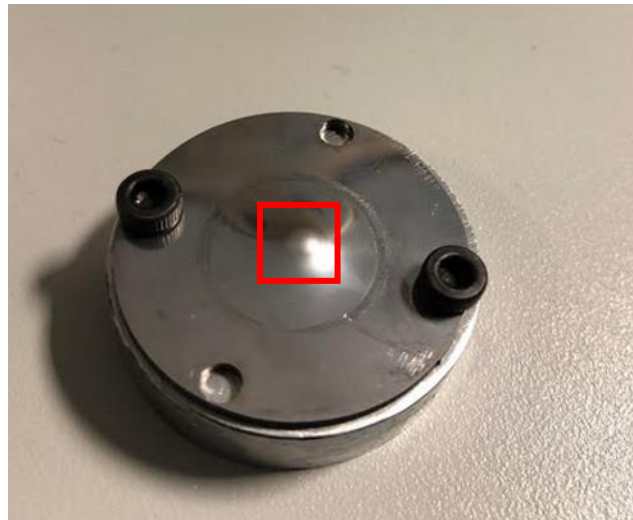
Fig. IX. 1 Sample after application of 2.6 mm displacement. Red square shows lack of visible crack on surface.
