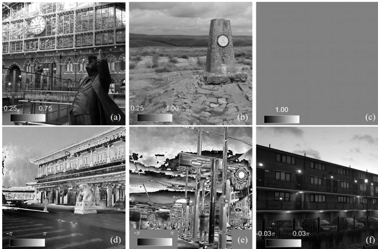
Figure 4. 6. The modulus and phase image of tested objects are shown in this figure. Each column is a modulus and phase pair of a tested object. The first row (i.e. (a) to (c)) demonstrates the modulus images of these objects, whereas the second row (i.e. (d) to (f)) demonstrates their phase images. To be more specific: the modulus (a) and phase (d) images of object for parameter optimisation, the modulus (b) and phase (e) images of strong object and the modulus (c) and phase (f) images of weak object. Each image comes with a colour bar to indicate their dynamic range. All images have the same size (3800×3800 pixels), which is large enough for all testing scenarios.
