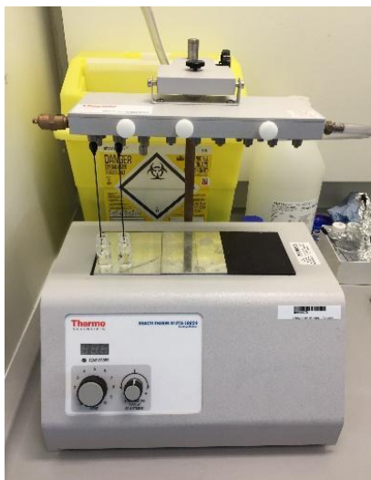
Figure 6. N 2 blow-down is set up in ENV 208 Fume Hood. Note 3 white plastic knobs near top. Each one can be used to isolate 9 blow-down positions if required and to control the amount of N 2 going to each tube.. Attach individual needles (the ones used only for CSIA) as required. There are blanking "screws" for positions not in use.
