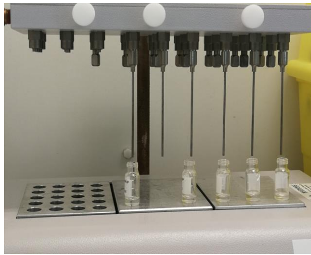
Figure 12. Samples transferred into GC vials then blown down under N_2 .
