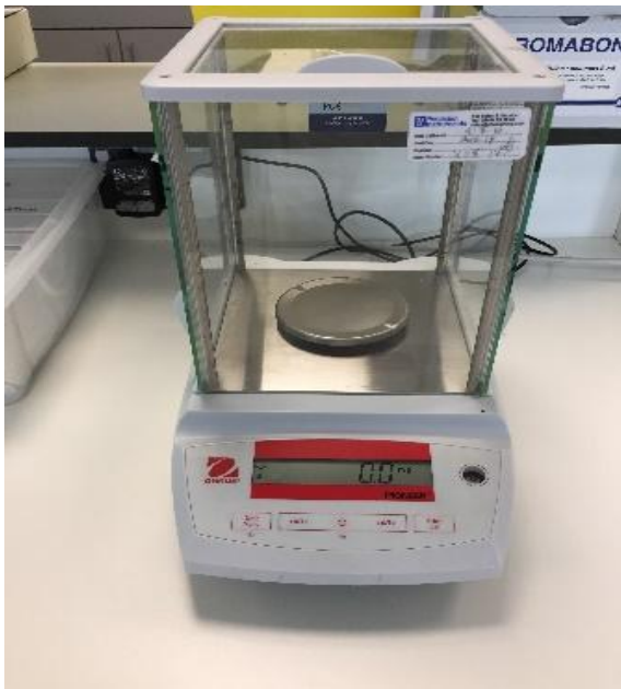
Figure 4. Use this balance (ENV/208) for weighing out samples and also for weighing exactly 5 mg of Norleucine.
