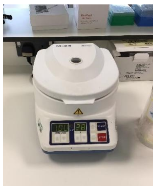
Figure 5. Use this centrifuge (facing the lab door; ENV208). Set speed to 100 and time to 1 min/60 s. Press start. (Ensure you have a balanced number of samples in the rotor).
