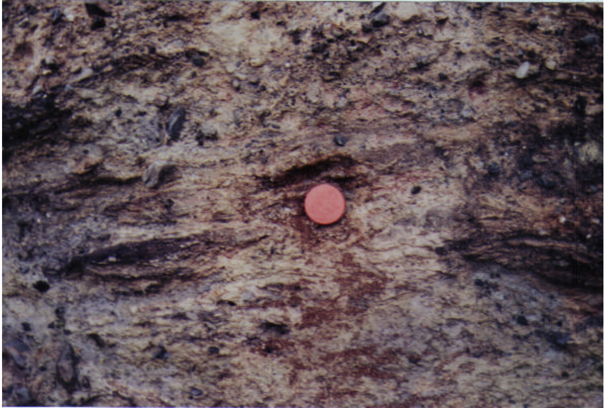
Figure 5.3 Interbedded sample area from the Criccieth deposit. Material is a mix of yellow and blue silts and clays, interbedded with short (~50 mm) sand lenses. Object in centre is a food tin lid ~7 cm.
