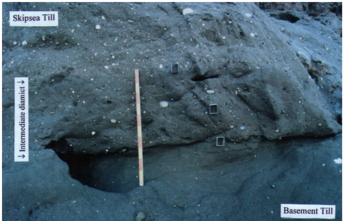
Figure 8.12 Photograph of the sediments sampled at the boundary between the Skipsea Till and the Basement Till at Dimlington High Ground, East Yorkshire coast. Open ended sample boxes are in the approximate sample positions.
