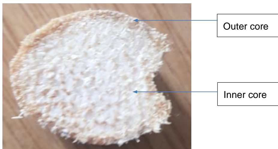
Figure 8.1 Transverse section of sorghum stalk residue (maximum diameter: 20 mm)
