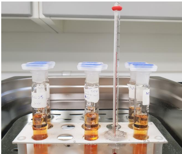
Figure 4.2 Placement of the unstable diesel-ethanol (DE) fuel blends within the temperature-controlled water bath
