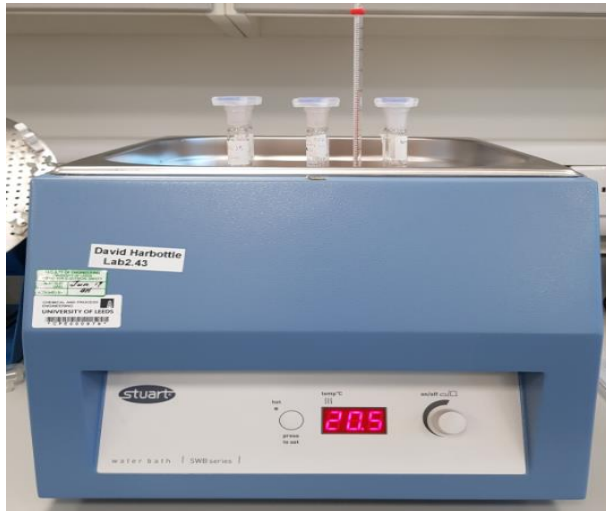
Figure 4.1 Experimental set up for the temperature sensitivity test of the unstable diesel-ethanol (DE) fuel blends
