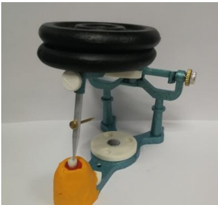
Figure 13 A constant weight of 1 kg was applied onto each restoration for 10 minutes until cement polymerisation was complete. The restorations were positioned in a standardised manner using an articulator where 1 kg weight was kept on the upper arm of the device.
