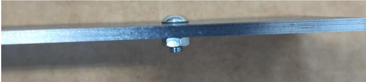
Figure 108 Side view of stack with new bolt arrangement prior to cutting
