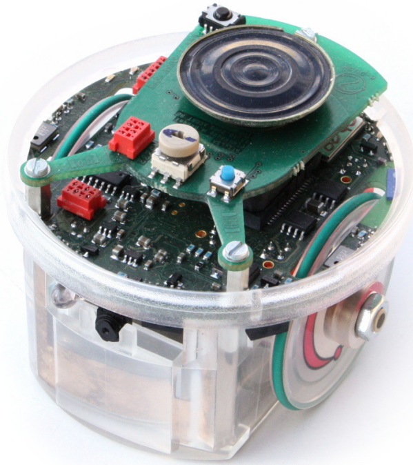
FIGURE 3.2: An e-puck robot. It has two differential wheels and a circular body with diameter 7.0 cm and height 4.5 cm, approximately. The robot is embedded with multiple sensory capabilities, for example, eight infrared proximity sensors and a VGA colour camera. Image used under the Creative Commons License.
