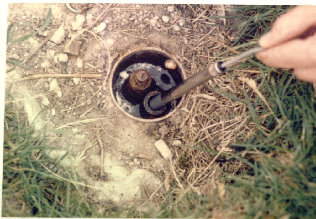
Plate No. 3.6 Measuring the elevation of the water table at Mam Tor.
