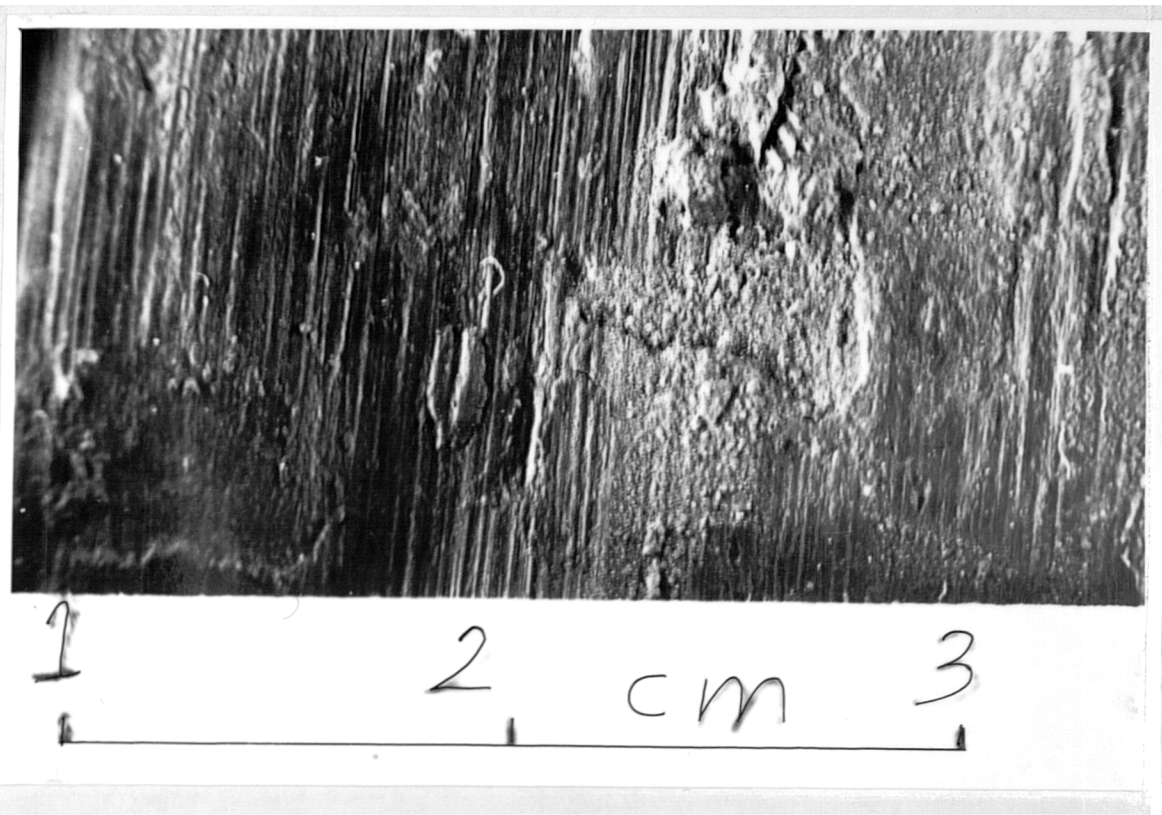
Plate No. 5.5 Slickensided shear surface - shear box test on sample SK.
