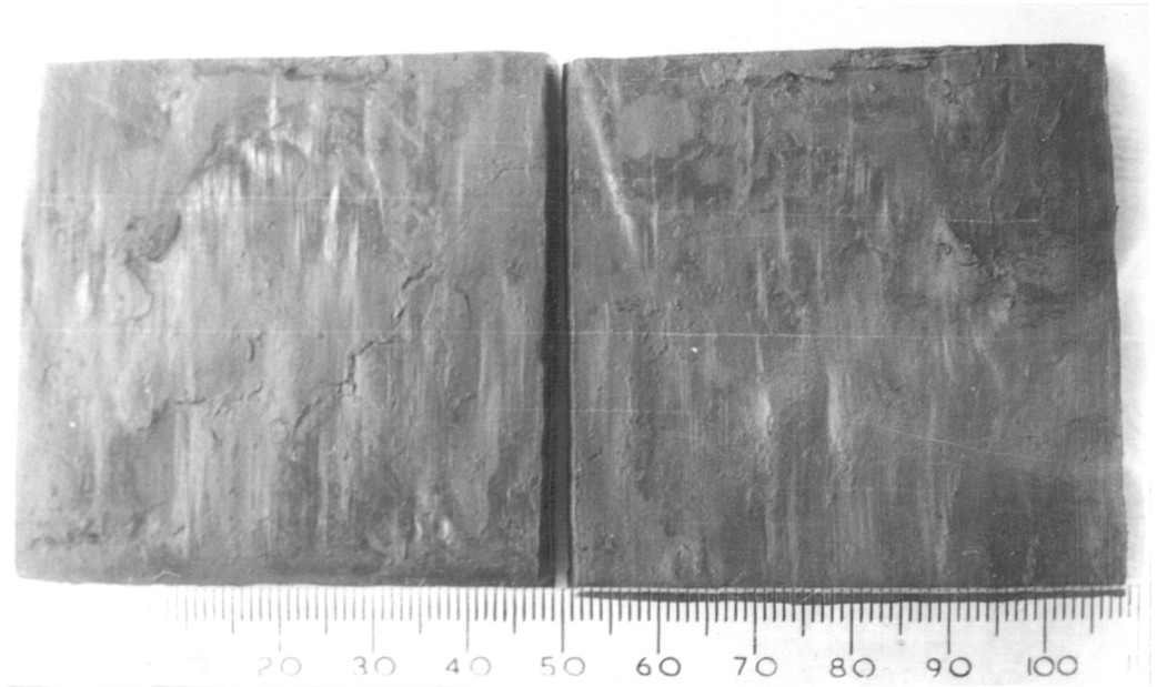
Plate No. 5.9 Slickensided shear surface - shear box test on sample MT5.
