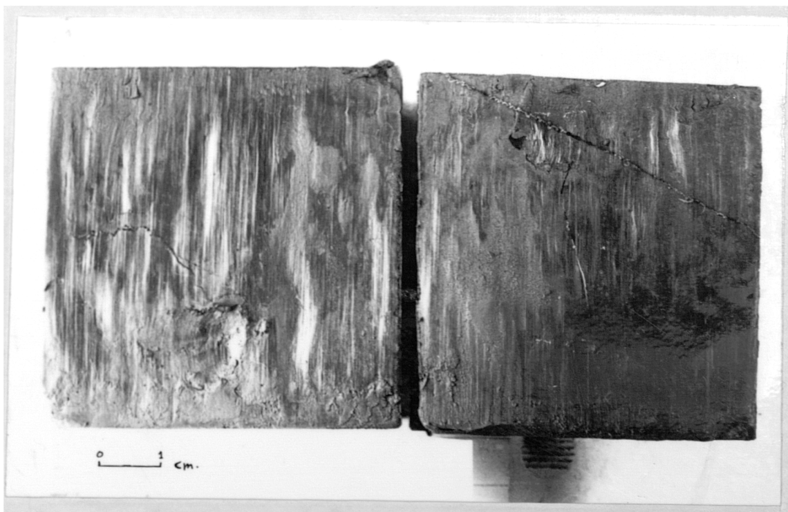
Plate No. 5.6 Slickensided shear surface - shear box test on sample CW1CP200.
