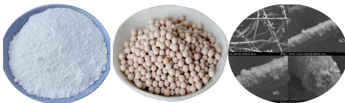
Figure 1.12. Typical forms of zeolite catalysts, powder (left), pellet (middle) and coating (right) on stainless steel [200]
